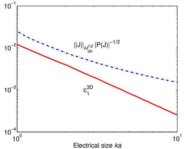
Fig. 2. Ratio of the Sobolev norm to the square root of the magnitude of the forward scattering amplitude for a plane wave induced current on a PEC sphere. The ratio is always bounded below by  $c_1^{3D}$ , as proved.
