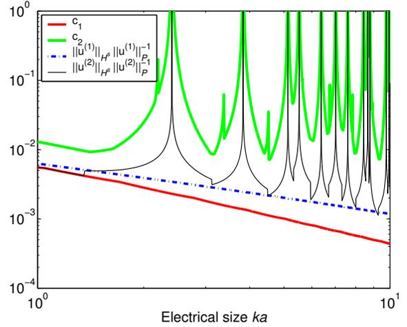
Fig. 1. Illustration of norm equivalence for two different test currents (TM polarization). The constants  $c_1$  and  $c_2$  always bound the ratio  $\|\cdot\|_{\mathcal{H}^s} / \|\cdot\|_P$ , which ratio is shown for the current induced by a plane wave ( $u^{(1)}$ ) and a nearest-to-resonance, single-mode current  $u^{(2)}$ . Similar results are obtained for the TE polarization.
