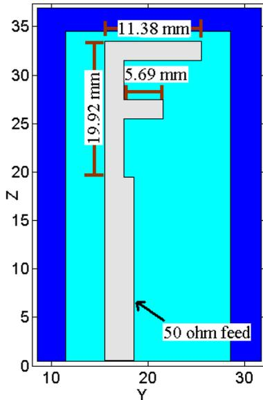
Fig. 1. Model of dual band 2.4/5.2 GHz “F” antenna as created by the authors.  $\Delta X = 0.762$  mm,  $\Delta Y = \Delta Z = 1.423$  mm. A ground plane on the back of the substrate extends from  $Z=1$  to the end of the 50 ohm feed at  $Z=19$ .
