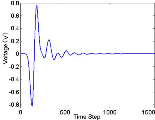
Fig. 3. Voltage on microstrip feed versus time.
