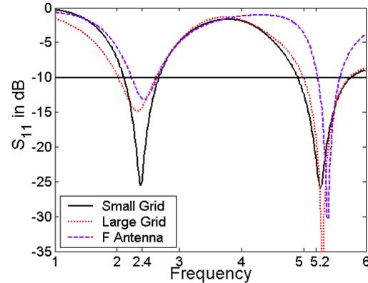
Fig. 8. Optimized  $S_{11}$  results as calculated on small grid (25x30x42 cells) for GA optimization, and large grid (100x100x100 cells) for comparison with “F” antenna. Even though the small grid introduces simulation error, the -10 dB bandwidth is very close on both simulations, justifying the use of the small grid for fast optimization.
