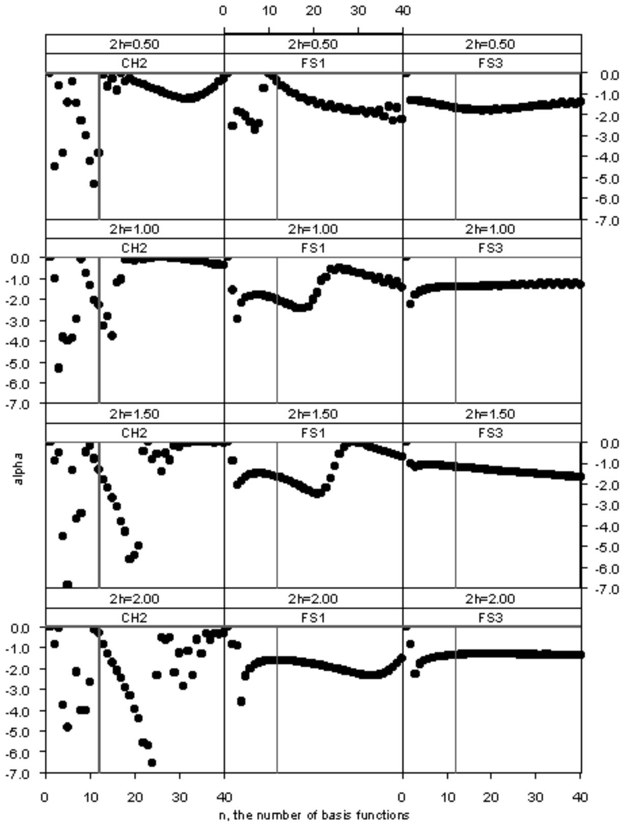
Figure 2a. Plots of alpha, for plane wave excitation, using the three main basis functions.
