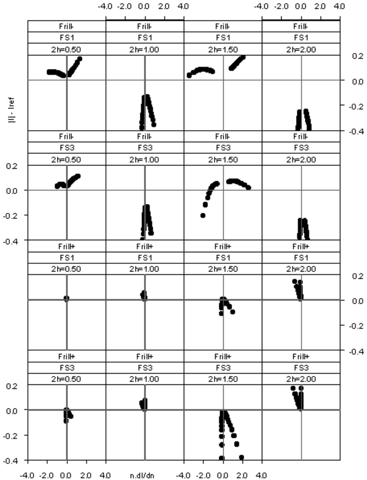
Figure 3. Scatter plots for dipoles of various lengths when excited by a magnetic frill with, Frill+, and without, Frill-, a special term representing the outgoing wave.
