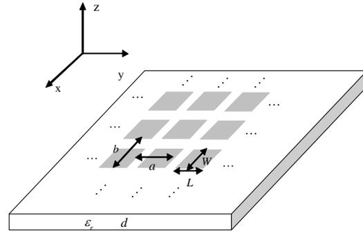
Fig. 11. The layout of the microstrip antenna.
