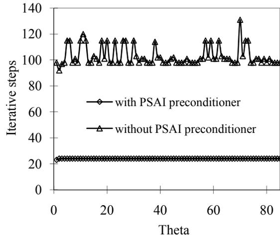
Fig. 13. The iterative steps of the LGMRES for the  $30 \times 30$  microstrip arrays simulated by the AIM with and without PSAI preconditioner,  $\varphi = 0^\circ$  and  $\theta$  is varying from  $0^\circ$  to  $85^\circ$ , and the frequency of the incident plane wave is 300MHz. And the tolerance of LGMRES is  $10^{-4}$ .
