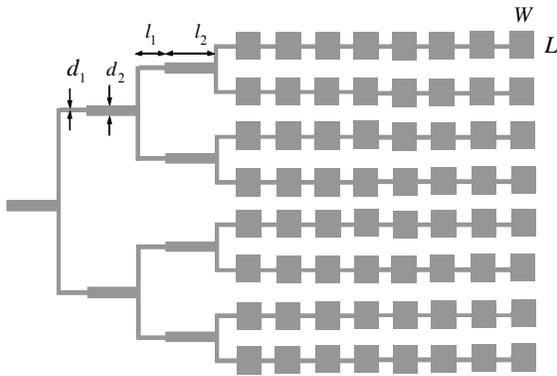
Fig. 7. The geometry of the  $8 \times 8$  microstrip corporate-fed planar antenna,  $L_1=12.32\text{mm}$ ,  $L_2=18.48\text{mm}$ ,  $W=10.08\text{mm}$ ,  $L=11.79\text{mm}$ ,  $d_1=1.3\text{mm}$ ,  $d_2=3.93\text{mm}$ , the thickness of substrate  $h=1.59\text{mm}$ ,  $\epsilon_r = 2.2$ .
