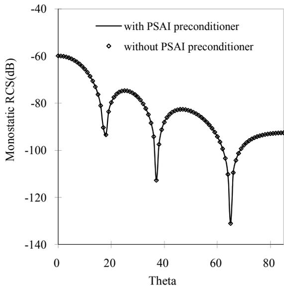
Fig. 12. The monostatic RCS of the  $30 \times 30$  microstrip arrays simulated by the AIM with and without PSAI preconditioner,  $\varphi = 0^\circ$  and  $\theta$  is varying from  $0^\circ$  to  $85^\circ$ , and the frequency of the incident plane wave is 300MHz.
