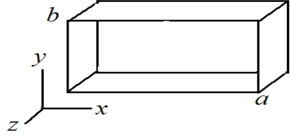
Fig. 1. Rectangular waveguide dimension reference.
