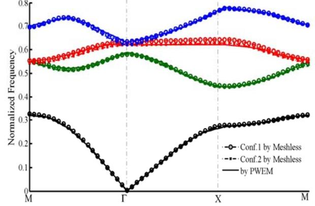
Fig. 5. Meshless results on band structures of square lattice composed of circular rods calculated by the periodic RPIM for two configurations (TM mode).
