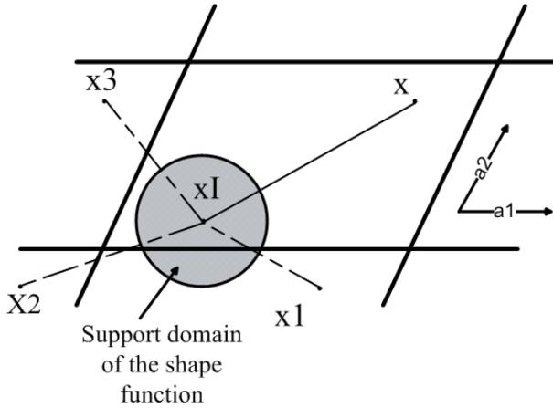
Fig. 1. A generic point in one of the shape function support domains in a unit cell. An actual point  $X$  and its three dual points, i.e.  $X_1$ ,  $X_2$ ,  $X_3$ , are shown. To determine the periodic shape function corresponding to  $X_i$  in point  $X$ , the shortest distance or the shortest line, i.e. dash line shown in the figure, must be used.
