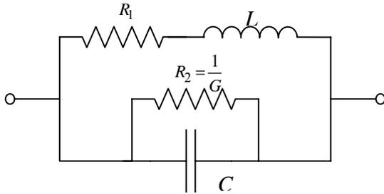
Fig. 3. Equivalent circuit for a second order rational function.
