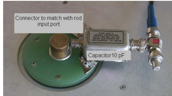
Fig. 2. Test setup of ECISM calibration method.
