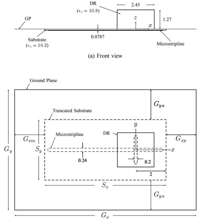
Fig. 12. RDRA with infinite ground plane. DR dimensions are  $2.45 \times 2.5 \times 1.27$ ; slot length is 1.8; microstripline input and stub lengths are 5.8 and 1.8 from center of slot, respectively;  $S_x = 8$  and  $S_y = 4$ , all in cm.
