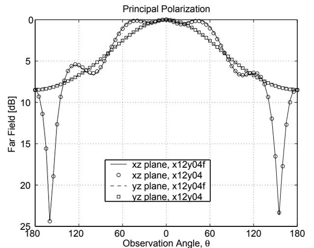
Fig. 13. Effect of substrate truncation of RDRA of Fig. 12 on radiation patterns with  $G_x = 12$ ,  $G_{xm} = 0$ ,  $G_{xp} = 4$ ,  $G_y = 4$ , all in cm. RDRA  $x12y04$  has truncated substrate as shown in 12, while  $x12y04f$  has full substrate.
