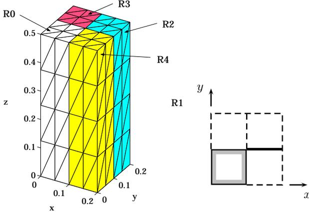
Fig. 8. Junction test case B — PEC block with three dielectric ones. Region R0 denotes conductor, and regions R2, R3, and R4 denote dielectric of  $\epsilon_r=2, 3,$  and  $4,$  respectively. The interface between R2 and R3 is dielectric, while that between R2 and R4 is PEC ( $\mathcal{PF}2$ ). PF0-Model in Fig. 9 treats surface of PEC block as  $\mathcal{PF}0$ , while PF2-Model treats it as  $\mathcal{PF}2$  with inside region being replaced by arbitrary dielectric. Units in m.
