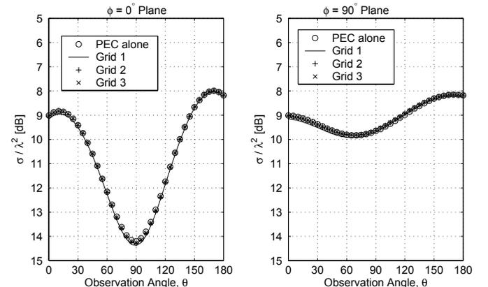
Fig. 7. RCS of T-junction with phantom dielectric.
