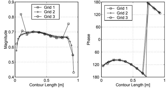
Fig. 6.  $\phi$ -directed magnetic currents of T-junction with phantom dielectric along circumferential contour ( $\phi = 0^\circ \rightarrow \phi = 180^\circ$ ,  $z = 0.0125$  m). Grid-1 and Grid-3 refer to grids shown in Figs. 3(b) and 5, respectively. Grid-2 is uniformly  $\phi$ -ne grid using 40 edges along the circumference.
