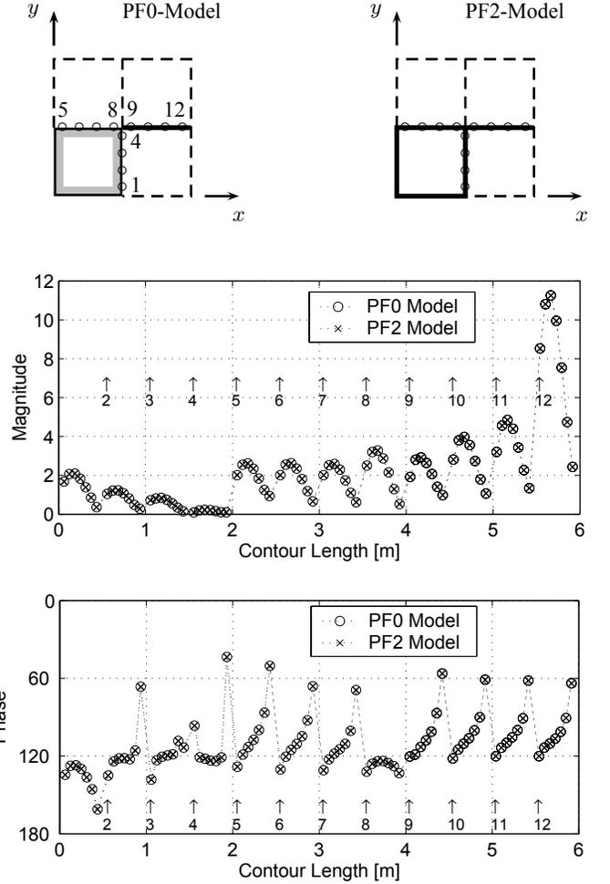
Fig. 9. Comparison of  $z$ -directed electric currents from two different models of PEC block shown in Fig. 8. Circles on geometry cross sections denote contour positions. Each contour runs from  $z = 0$  to  $z = 0.5$ .
