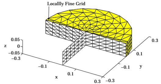
Fig. 5. Modeling with locally  $\phi$ -ne grids (Grid-3).
