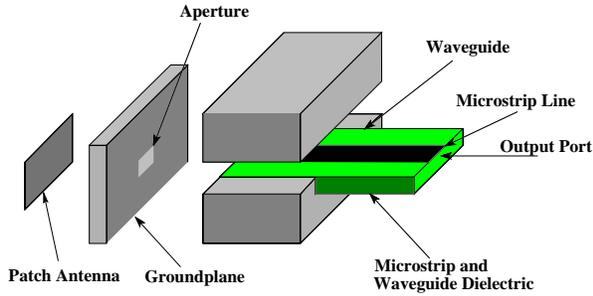
Fig. 5. A rectangular patch antenna coupled through slot to a waveguide-to-microstrip line junction.
