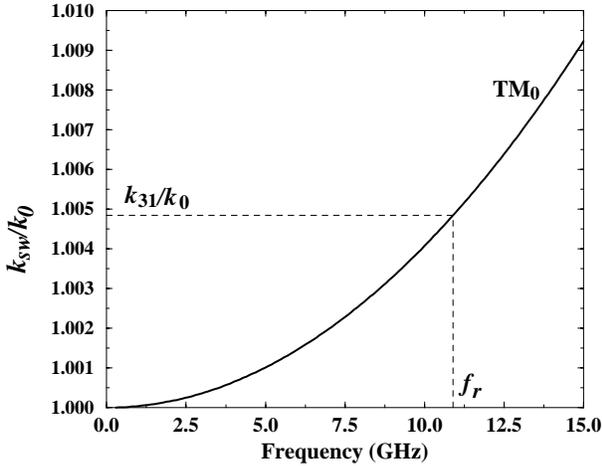
Fig. 9. Dispersion behavior of the normalized propagation constant of the dominant  $TM_0$  mode in a grounded dielectric slab waveguide.
