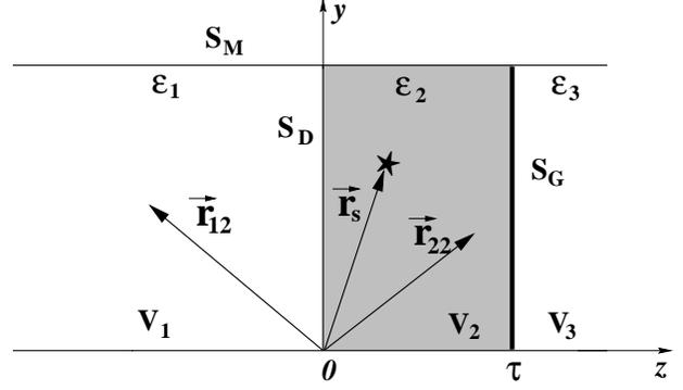
Fig. 3. Two-layered, terminated rectangular waveguide with an electric point source (starred) arbitrarily located in region  $V_2$  used in the magnetic-field formulation.
