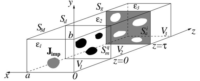
Fig. 1. Waveguide-based transition module of interacting electric- (patch, strip) and magnetic-type (slot, aperture) discontinuities.
