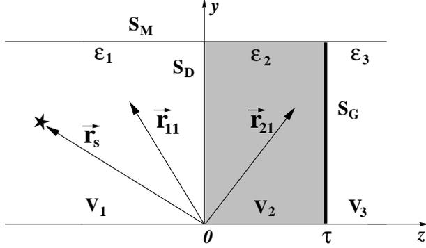
Fig. 2. Two-layered, terminated rectangular waveguide with an electric point source (starred) arbitrarily located in region  $V_1$  used in the electric-field formulation.
