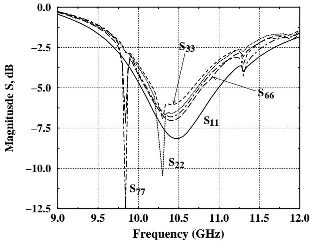
Fig. 11. Magnitude of the reflection coefficients versus frequency for the  $3 \times 4$  aperture-coupled patch array in the 13-port rectangular waveguide transition.
