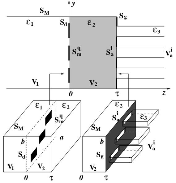
Fig. 4. A waveguide-based aperture-coupled patch array in the  $N$ -port waveguide transition.
