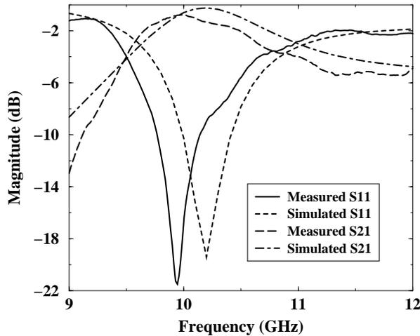
Fig. 6. Numerical and experimental results for the reflection and transmission coefficient of the single unit cell, including a waveguide-based aperture-coupled patch antenna and a waveguide-to-microstrip line junction.
