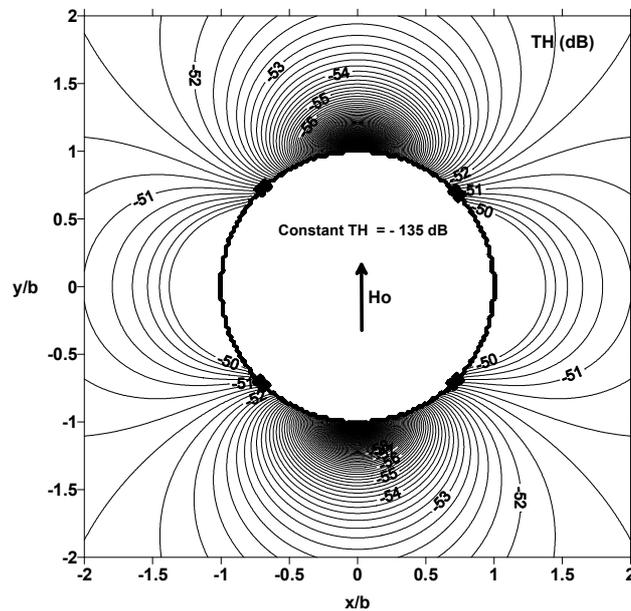
Figure 7. Contour plot of the total H-field transfer function (in dB) in the equatorial plane, inside and outside the aluminum shell, for  $b = 0.914$  m,  $\Delta = 0.794$  mm, and  $f = 100$  kHz.
