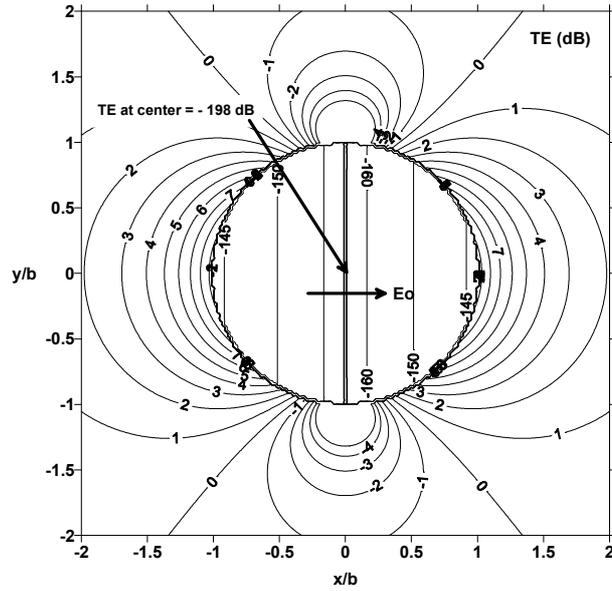
Figure 6. Contour plot of the total E-field transfer function (in dB) in the equatorial plane, inside and outside the aluminum shell, for  $b = 0.914$  m,  $\Delta = 0.794$  mm, and  $f = 100$  kHz.
