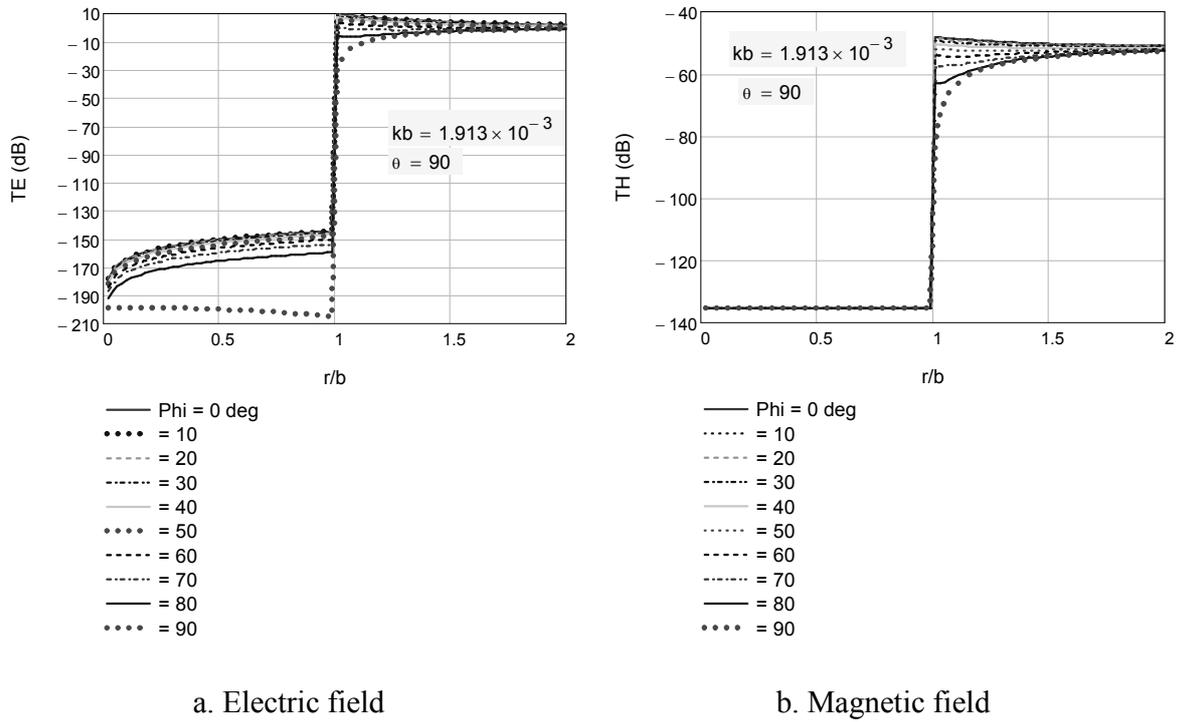
**Figure 5.** Plots of the total E- and H-field transfer functions in the equatorial ( $z = 0$ ) plane along different trajectories defined by the angle  $\phi$ . (Parameters are  $b = 0.914$  m,  $\Delta = 0.794$  mm, and  $f = 100$  kHz.)
