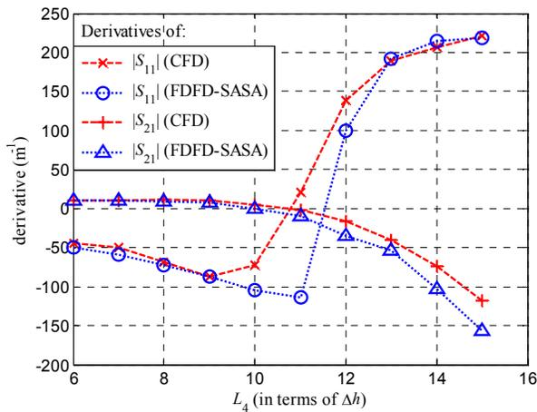
Fig. 3. Derivative curves for the  $S$ -parameter magnitudes of a waveguide filter calculated from field solutions obtained from a simulation with Ansoft HFSS. The plot validates our results (marked FDFD-SASA) with response-level central finite differences (marked CFD). Derivatives are with respect to a shape parameter  $L_4$  for a sweep of  $L_4$ .
