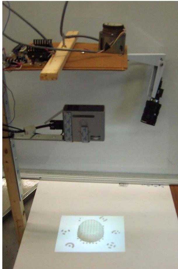
Fig. 8. Photogrammetry system for surface shape acquisition. The knowledge of the shape of the object whose interior is imaged through microwave  $S$ -parameter measurement enhances greatly the speed and the convergence of the reconstruction algorithm.
