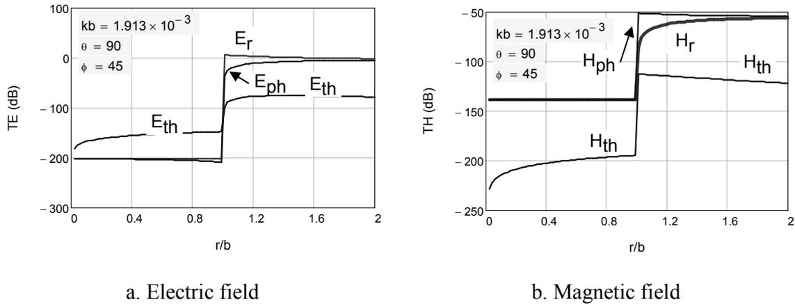
**Figure 4. E- and H-field transfer functions for the  $r$ ,  $\theta$  and  $\phi$  field components for the spherical shell of inner radius  $b = 0.914$  m and shell thickness  $\Delta = 0.794$  mm, at a frequency of 100 kHz. (These E-fields are shown as a function of radial distance on a path defined by the angles  $\theta = 90^\circ$  and  $\phi = 45^\circ$ .)**
