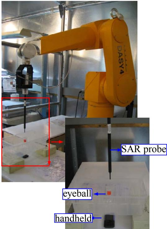
Fig. 9. SAR measurement robot with our human-eye phantom.
