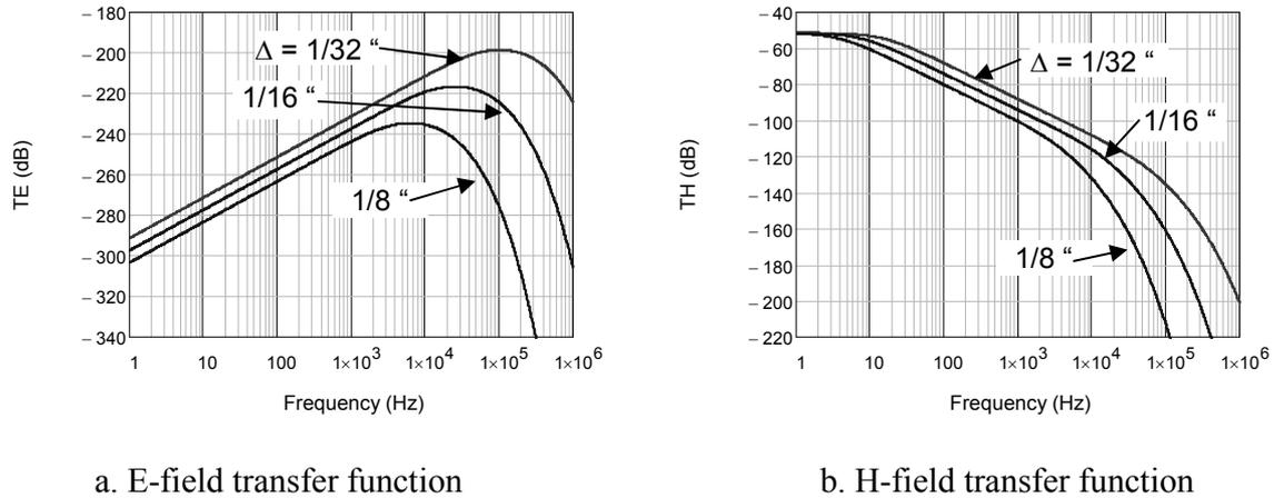
**Figure 2.** Plots of the total E-field and H-field transfer functions at the center of an aluminum sphere with radius  $a = 0.914$  m for different shell thicknesses,  $\Delta$ . (To be compared with Figures 2 and 8 of ref. [8].)
