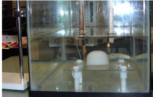
Fig. 4.  $S$ -parameter measurement of a breast phantom.
