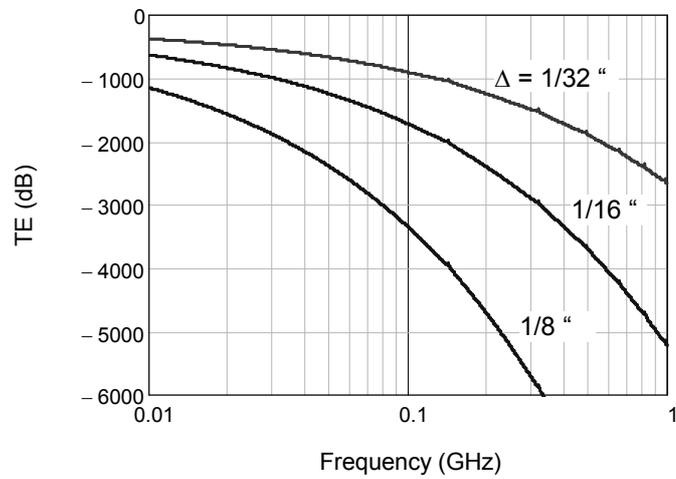
a. TE for three different shell thicknesses.
