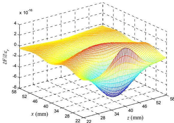
Fig. 2. Permittivity Jacobian map at 4 GHz in an  $x$ - $z$  cross-section of a breast model derived from a time-domain field solution obtained with Quickwave-3D. The minimum indicates the presence of a small scatterer (tumor simulant).
