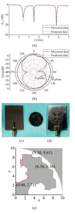
Fig. 8. Optimization results for the example and photograph of the fabricated antenna: (a)  $|S_{11}|$ , (b) radiation patterns at the first resonant frequency, (c) top view, (d) back view, (e) image of a quarter of slot.
