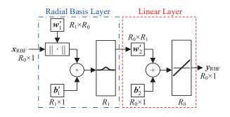
Fig. 4. Structure of the radial basis function network.
