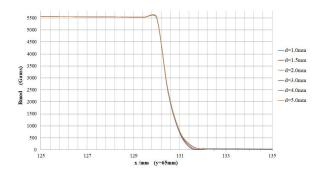
Fig. 2. Leakage magnet field with different septa.
