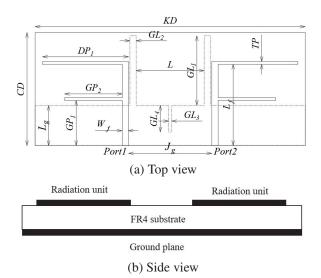
Fig. 6. Configuration of the dual-band MIMO antenna for WLAN (KD = 63 mm, CD = 28 mm,  $W_f = 1.4 \text{ mm}$ ,  $L_f = 18 \text{ mm}$ ,  $GP_1 = 9 \text{ mm}$ ,  $J_g = 18.5 \text{ mm}$ ,  $L_g = 8.9 \text{ mm}$ ,  $GL_2 = 1.4 \text{ mm}$ ,  $GL_4 = 5.9 \text{ mm}$ , L = 15.1 mm).
