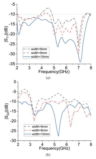
Fig. 4. The width evolution of the proposed antenna: (a)  $S_{11}$  and (b)  $S_{22}$ .
