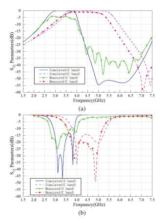
Fig. 3. Comparisons between simulated and measured results: (a)  $S_{21}$  parameters and (b)  $S_{11}$  parameters.
