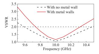
Fig. 8. Simulated VSWR of the center elements.
