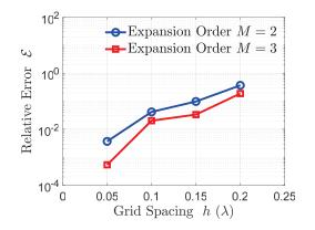
Fig. 10. Relative errors  $\mathscr{E}$  of the surface currents coefficients with respect to different grid spacings h and expansion orders M. The relative errors of the proposed PSG-FFT-ACA algorithm are illustrated. The surface currents coefficients obtained using the standard MoM are used as the reference.
