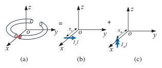
Fig. 4. Equivalent model of a circular arc antenna: (a) Circular arc antenna with angle  $\Phi$ , (b) electric dipole  $I_e l$ , and (c) magnetic dipole  $I_m l$ .
