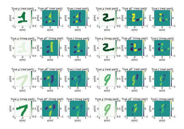
Fig. 3. Examples of the branch network input  $\overline{\overline{\chi}} \oplus \overline{\overline{\chi}} \circ \overline{\overline{E}}^i$  and corresponding equivalent electric current labels.
