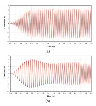
Fig. 8. Induced current across the load of the Rx coil (separation distance equals 4 cm, time-harmonic excitation at 13.56 MHz): (a) optimum load and (b) 50  $\Omega$  load.
