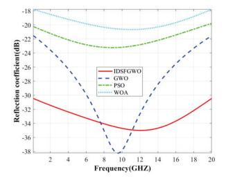
Fig. 7. Reflective coefficient curve of 7-layers design.
