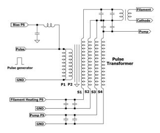
Fig. 2. Detailed circuit of pulse transformer application.
