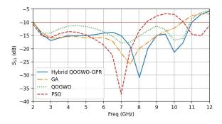
Fig. 4. Comparison of  $S_{11}$  curves from different algorithms.
