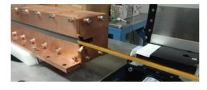
Fig. 9. Point coil for measuring the end field.
