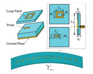
Fig. 3. Structure of the 12-element TCCA, with top, back, and cross-sectional views of the planar surface.
