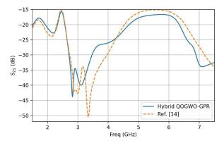
Fig. 9. Comparison of  $S_{21}$  curves between Ref. [14] and the hybrid algorithm.
