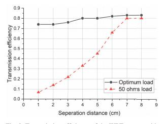
Fig. 9. Transmission efficiency of the WPT system with the optimum load and 50  $\Omega$  load.
