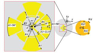
Fig. 7. The phototype of the C-shaped monopole (design parameters [millimetres]: R1 = 9, R2 = 16, R3 = 10, R4 = 8.5, R5 = 21, R6 = 7, R7 = 16, Rd1 = 6.5, Rd2 = 7.5, w = 1.3, d = 2, g = 0.5, Wd = 2.3).
