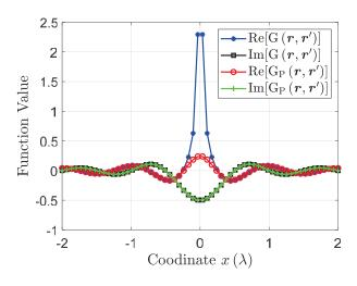
Fig. 3. The function values of  $G(\mathbf{r}, \mathbf{r}')$  and  $G_P(\mathbf{r}, \mathbf{r}')$ . The source point  $\mathbf{r}'$  is fixed to the coordinate origin, and the field point  $\mathbf{r}$  is moving along the *x* axis.
