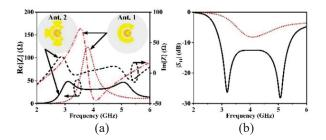
Fig. 5. The performance of two C-shaped monopoles: (a) Impedance, (b)  $|S_{11}|$ .
