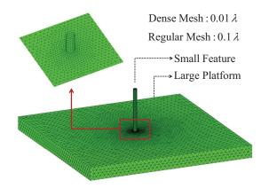
Fig. 9. Mesh configurations of a small monopole antenna on top of a large platform. A multiscale mesh is used to discretize this object. The monopole antenna is discretized using dense mesh of about 0.01  $\lambda$ , while the large platform is discretized with regular mesh of about 0.1  $\lambda$ .
