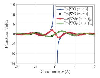
Fig. 4. The function values of  $[\nabla G(\mathbf{r},\mathbf{r}')]_x$  and  $[\nabla G_P(\mathbf{r},\mathbf{r}')]_x$ . The source point  $\mathbf{r}'$  is fixed to the coordinate origin, and the field point  $\mathbf{r}$  is moving along the *x* axis.
