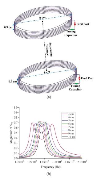
Fig. 1. (a) Structural diagram of the WPT system, and (b) power transfer efficiency versus the separation distance between the Tx and Rx coils.
