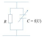
Fig. 5. The proposed realization of the optimum load.
