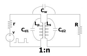
Fig. 1. A typical pulse transformer circuit. V is the source of the ideal pulse, r is resistance of pulse source,  $C_{d1}$  and  $C_{d2}$  are winding line distribution capacity,  $C_w$  is stray capacitance between primary and secondary windings,  $L_p$  and  $L_s$  are primary and secondary inductance, R is load.
