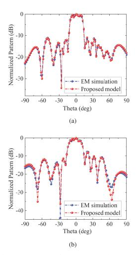
Fig. 4. Pattern results of the proposed model and the fullwave simulation at 3.5 GHz: (a) Array 1 and (b) Array 2.
