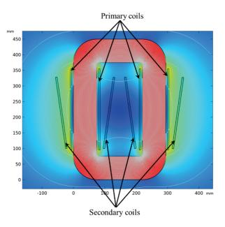
Fig. 7. Magnetic flux density of the designed pulse transformer.
