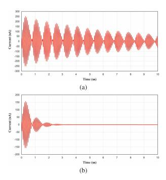
Fig. 7. Induced current across the load of the Rx coil (separation distance equals 4 cm, unit pulse is applied): (a) optimum load and (b) 50  $\Omega$  load.
