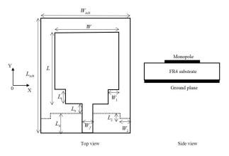
Fig. 2. Configuration of the stepped ultrawideband monopole antenna ( $W_{sub} = 20 \text{ mm}$ ,  $L_{sub} = 30 \text{ mm}$ , W = 16 mm, L = 18 mm,  $L_4 = 5 \text{ mm}$ ).
