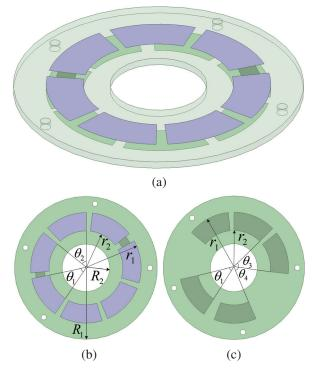
Fig. 1. Antenna geometry structure: (a) top view, (b) upper layer, and (c) bottom layer.
