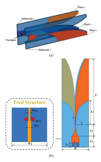
Fig. 3. Geometry of a BAVA without slots: (a) 3D view and (b) 2D view.
