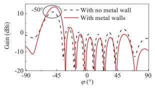
Fig. 10. Radiation patterns of arrays at 10 GHz in the *xoy*-plane with  $\varphi = -50^{\circ}$ .
