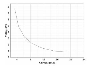
Fig. 4. V-I curve of the optimum load.
