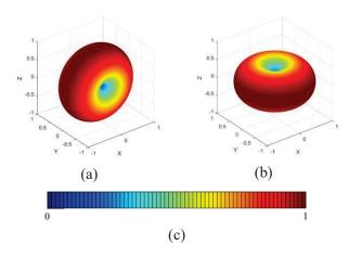
Fig. 5. Radiation patterns of (a) an electric dipole along the y direction and (b) a magnetic dipole along the z direction; (c) the color map.
