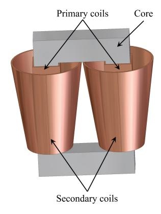
Fig. 4. 3D view of the pulse transformer structure.
