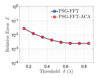
Fig. 8. Relative errors  $\mathscr{E}$  of the surface currents coefficients I with respect to different splitting threshold  $\delta$ . The relative errors of both the traditional PSG-FFT algorithm and the proposed PSG-FFT-ACA algorithm are illustrated. The surface currents coefficients obtained using the standard MoM are used as the reference.
