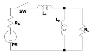
Fig. 6. Equivalent circuit for leading edge analysis.
