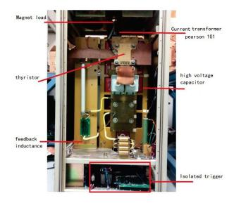
Fig. 8. Layout of excitation pulse power supply.
