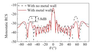
Fig. 7. Monostatic RCS of the array at 12 GHz.
