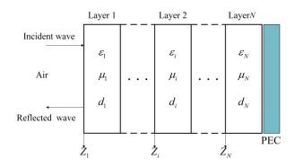
Fig. 1. Structure of multilayer microwave absorber.
