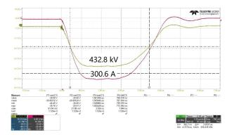
Fig. 11. Output waveform of the pulse transformer.
