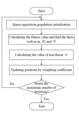
Fig. 1. The flowchart of the QOGWO algorithm.
