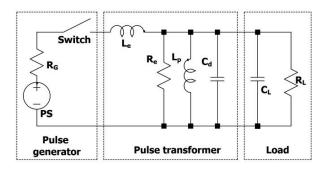
Fig. 5. Equivalent circuit model of the pulse transformer.  $R_G$  means the impedance of power supply,  $L_e$ indicates the leakage inductance,  $R_e$  means equivalent impedance of eddy current loss,  $L_P$  is the primary coil inductance,  $C_d$  is stray capacitance between coils and grand,  $C_L$  means the load stray capacitance, and  $R_L$  means impedance at primary side.
