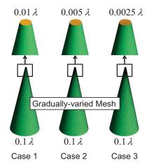
Fig. 11. Mesh configurations of the PEC cone. A gradually-varied mesh is used to discretize the coneshape object. The edge length for the regular part of the mesh is 0.1  $\lambda$ . The edge lengths for the dense part of the mesh are 0.01  $\lambda$ , 0.005  $\lambda$ , and 0.0025  $\lambda$ , respectively. For clarity, the enlarged views are also shown in the above.
