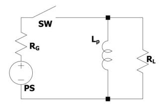
Fig. 8. Equivalent circuit for flat-top droop analysis.
