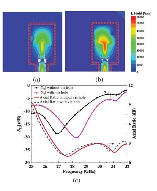
Fig. 5. (a) Electric field distribution without via hole, (b) electric field distribution with via hole, and (c) simulated  $|S_{11}|$  and axial ratio in both (a) and (b) cases.
