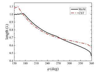
Fig. 11. Length of circular arc antenna with different angles when the arc antenna is the closest to near isotropic radiation.
