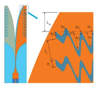
Fig. 4. Geometry of the curved slots.
