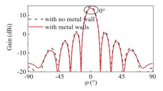
Fig. 9. Radiation patterns of arrays at 10 GHz in the *xoy*-plane with  $\varphi = 0^{\circ}$ .
