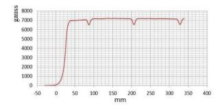
Fig. 10. Field distribution along beam direction.
