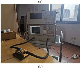
Fig. 4. (a) Fabricated filter and (b) test platform.
