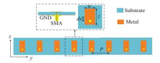
Fig. 2. Structure of the array with no metal wall, where dx = 2.4 mm, w = 6.5 mm, and l = 8.3 mm.
