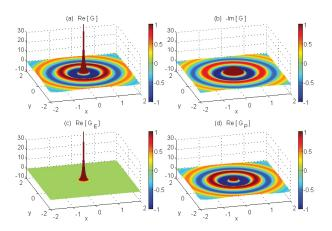
Fig. 1. The Green's function is a priori split into a singular but spatially localized part  $G_E$  and a globally oscillatory but spectrally band-limited part  $G_P$ . The relevant magnitudes of the original Green's function and of these two parts are visualized in the figure.
