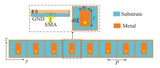
Fig. 5. Structures of the array with metal walls.
