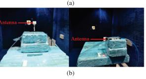
Fig. 6. Fabricated prototype of the CP antenna: (a) Prototype with connectors installed and (b) antenna under test in the anechoic chamber.
