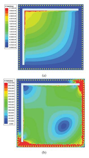
Fig. 2. Field plot: (a) Electric field distributions of a quarter DFSIW cavity and (b) magnetic field distributions of a quarter DFSIW cavity.
