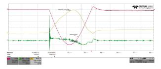
Fig. 13. Induced voltage and integration of leakage field.
