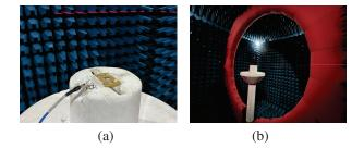
Fig. 11. The antenna in anechoic chamber.
