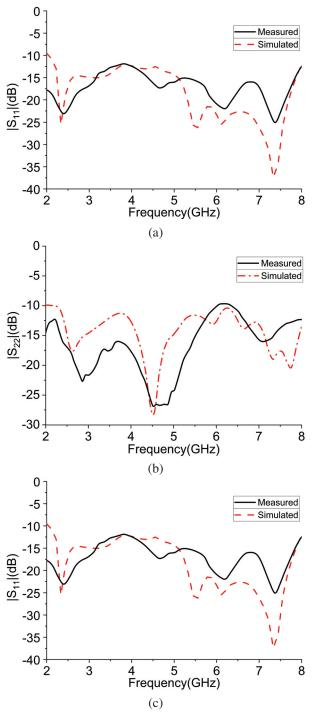
Fig. 7. Simulated and measured *S*-parameters of the proposed antenna: (a)  $S_{11}$ , (b)  $S_{22}$ , and (c)  $S_{12}$ .
