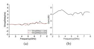
Fig. 9. (a) Measured group delay and (b) measured peak gains.
