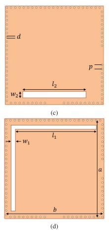
Fig. 1. Design structure of the filter: (a) 3-D view, (b) the top view of feed part, (c) couple layer, and (d) the top view of a DFSIW resonator.
