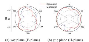
Fig. 8. The radiation patterns of (a) *E*-plane and (b) *H*-plane at 5.5 GHz.
