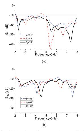
Fig. 3. The evolution of the proposed antenna: (a)  $S_{11}$  and (b)  $S_{22}$ .
