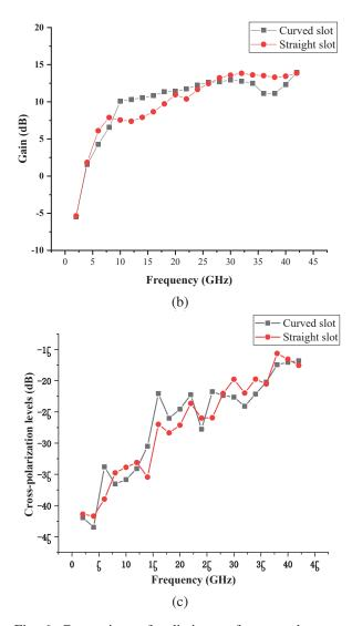
Fig. 6. Comparison of radiation performance between BAVAs with curved slots and straight slots: (a)  $|S_{11}|$ , (b) gain, and (c) cross-polarization level.
