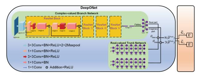
Fig. 2. The overall flow of employing the DeepONet to solve EM scattering problems.
