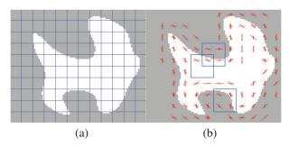
Fig. 3. Extraction of histogram of oriented gradients features: (a) Binary image Z with cells, (b) visualization of the histogram of oriented gradients feature and blocks.
