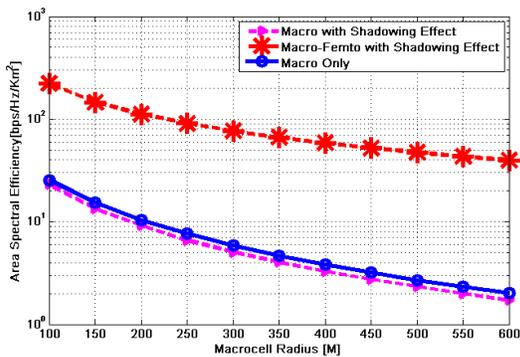
Fig. 2. Effect of shadowing on the area spectral efficiency for  $\sigma_d = 4$  dB.
