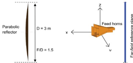
Fig. 6. A parabolic and two overlapped feed horns.
