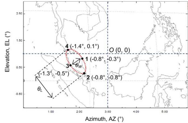
Fig. 7. Illustration showing the beam coverage for B<sub>1</sub> region with the -3 dB EOC points.
