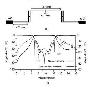
Fig. 5. Two cascaded resonators: (a) schematic, and (b) simulation.
