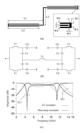
Fig. 1. Basic resonator: (a) layout, (b) LC model, and (c) frequency responses.
