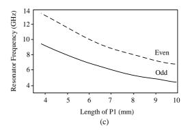
Fig. 3. (a) The configuration of the dual-mode microstrip resonator, (b) simulated resonances of the two modes against P2, and (c) simulated resonances of the two modes against P1.
