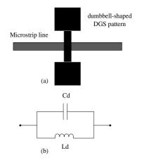
Fig. 6. DS-DGS: (a) layout, and (b) LC model.
