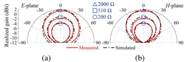
Fig. 10. The radiation patterns of the antenna prototypes at 5.8 GHz: (a) E-plane and (b) H-plane.
