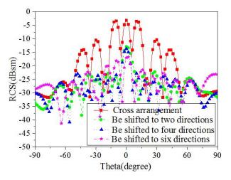
Fig. 7. 2D far-field scattering pattern plotted in y-z plane.
