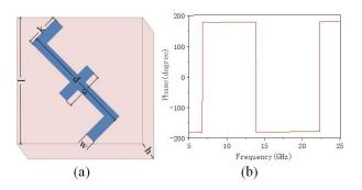
Fig. 4. (a) Structure diagram of polarization conversion unit. (b) Cross-polarization phase difference.
