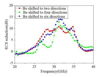
Fig. 9. Simulation results of RCS reduction.
