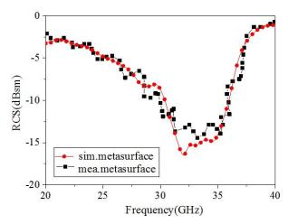
Fig. 11. Comparison of single-station RCS results of metasurface under normal incident of electromagnetic wave.
