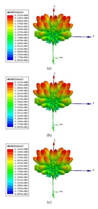
Fig. 6. The cross-arrangement scattering patterns are shifted to multiple directions at f = 32GHz.
