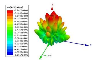
Fig. 5. The cross-arrangement scattering pattern at f = 32GHz.
