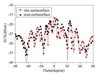
Fig. 12. Comparison of 2D far-field scattering pattern of metasurface under normal incident of electromagnetic wave.
