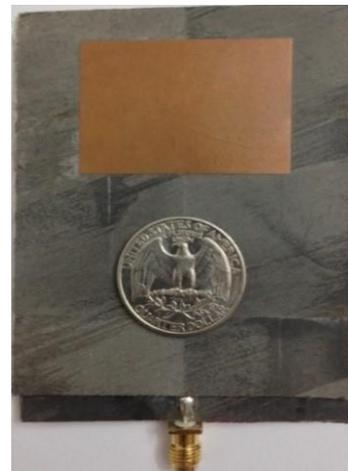
Fig. 6. Top view of the fabricated antenna.
