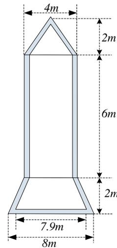
Fig. 3. Geometry structure of a PEC missile model.
