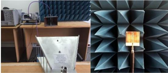
Fig. 9. Measurement setup for maximum far field gain.
