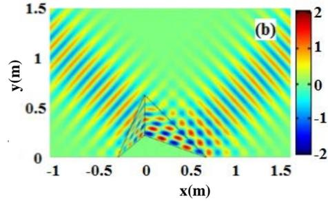
Fig. 4. A lateral view of the invisibility cloak designing procedure corresponding to the particular case in which  $x_N = x_M$ . (a) 2D design of triangular bump covered with the ground cloak of simpler designing relations. (b) Electric field distribution of a TE-polarized Gaussian beam incident incoming from left at an azimuth angle of  $45^\circ$  on the cloaked bump at the frequency of 2 GHz.
