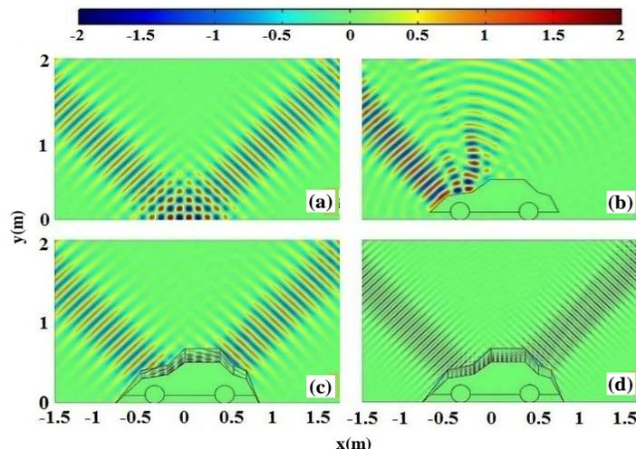
Fig. 6. The electric field distribution of a Gaussian beam incident under TE-polarization incoming from left at an azimuth angle of  $45^\circ$  on: (a) flat PEC ground plane, (b) contour cross section of a schematic car (0.5 m height and 1.5 m length) with the PEC outer surface, (c) and (d) the 2D designed ground invisibility cloak for the schematic car contour of Fig. 6 (b), at 2 GHz and 5 GHz, respectively.
