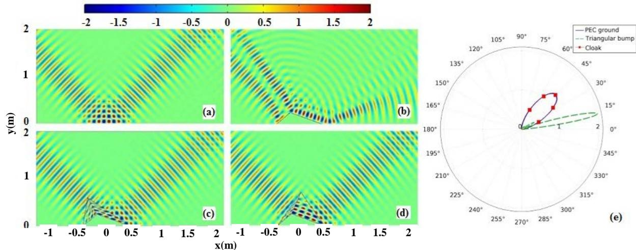
Fig. 2. The electric field distribution of a TE-polarized Gaussian beam incident from the left with  $45^\circ$  azimuth angle on: (a) flat PEC ground plane, (b) triangular PEC bump with 0.25 m height and 0.5 m base, (c) and (d) 0.5 m height designed cloaks for the triangular bump depicted in Fig. 2 (b), (e) Normalized average power outflows corresponding to Figs. 2 (a)-(d).
