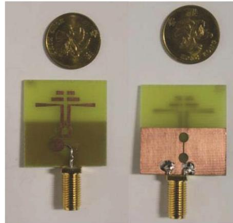
Fig. 5. Fabricated prototype of the proposed antenna.
