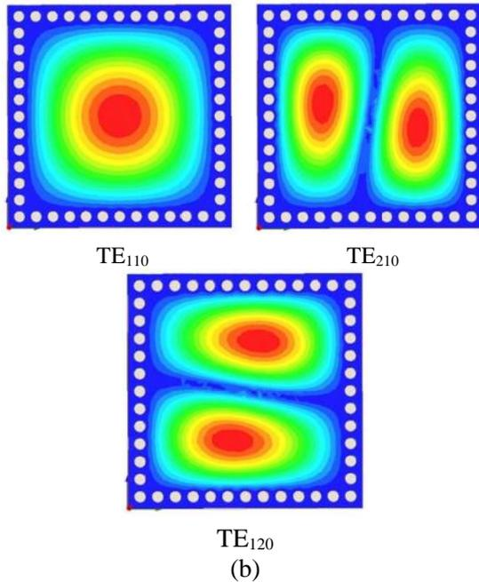
Fig. 1. (a) Geometry of a square cavity, and (b) electric field distribution at three first modes.
