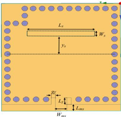
Fig. 4. Single element antenna structure.
