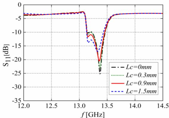
Fig. 7. Simulation results of  $S_{11}$  for the proposed array versus frequency and different values of  $L_c$ .
