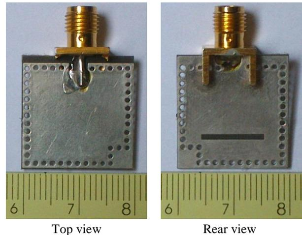
Fig. 8. Photo of the fabricated proposed single element antenna.
