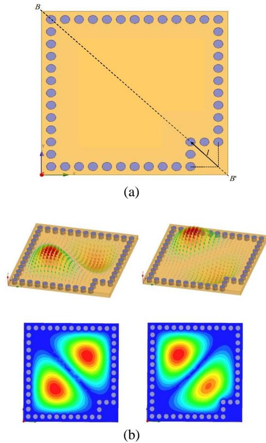
Fig. 2. (a) Geometry of the perturbed square cavity, and (b) simulated electric field distribution at  $TE_{210}$  and  $TE_{120}$ .
