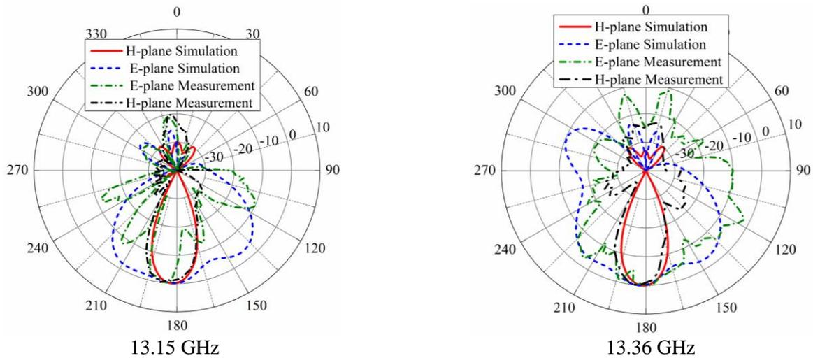
Fig. 14. Measured and simulated radiation patterns of the antenna array at two frequencies.
