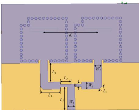
Fig. 6. Two elements antenna array.
