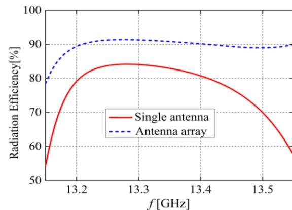
Fig. 13. Simulated radiation efficiency of the proposed single and antenna array.
