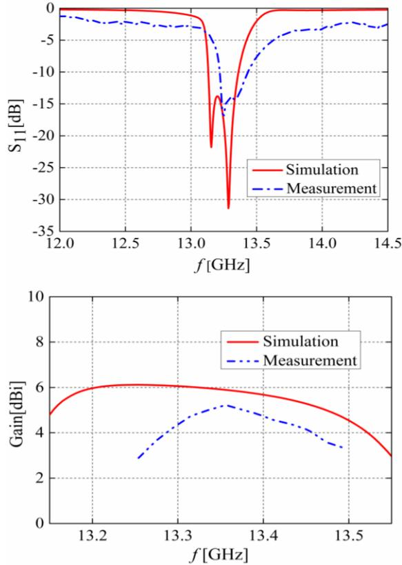
Fig. 9. Measured and simulated results of the single element antenna at boresight direction of: (a)  $S_{11}$ , and (b) gain.
