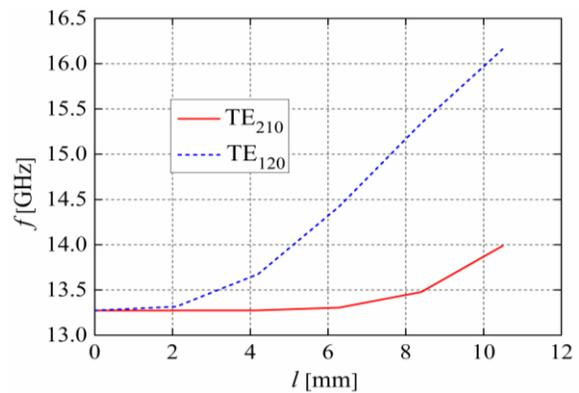
Fig. 3. Variation of the simulated resonate frequency of the degenerate modes versus perturbation size  $l$ .
