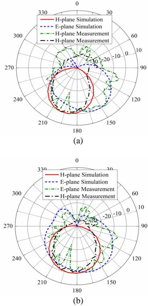
Fig. 10. Measured and simulated radiation patterns of the single antenna at: (a) 13.15 GHz, and (b) 13.29 GHz.
