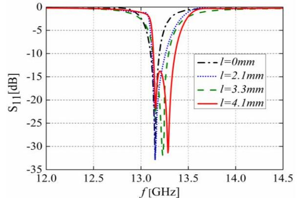
Fig. 5. Simulation results of  $S_{11}$  versus frequency for a perturbed cavity and different values of  $l$ .
