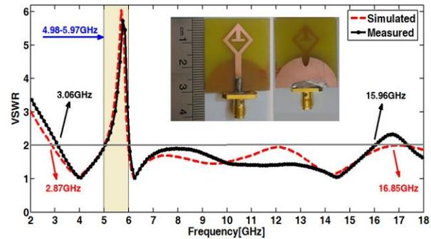
Fig. 11. Measured and simulated VSWR of the proposed optimized antenna. Inset is the photograph of the front and back side of the antenna.
