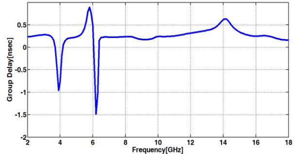
Fig. 10. Measured group delay of the proposed antenna.
