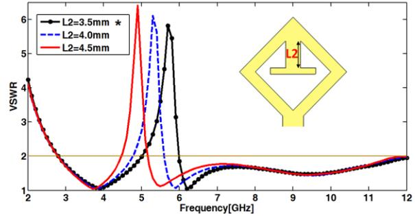
Fig. 6. Simulated VSWR characteristics of the proposed antenna for various dimensions of parameter  $L_2$ .
