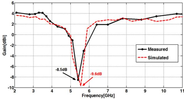
Fig. 8. Measured and simulated gain of the antenna.
