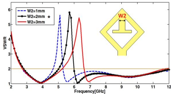
Fig. 4. Simulated VSWR characteristics of the proposed antenna for various dimensions of parameter  $W_2$ .
