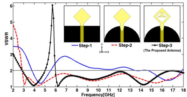
Fig. 2. Simulated VSWR characteristic of the antenna in the various steps to create the final proposed structure.
