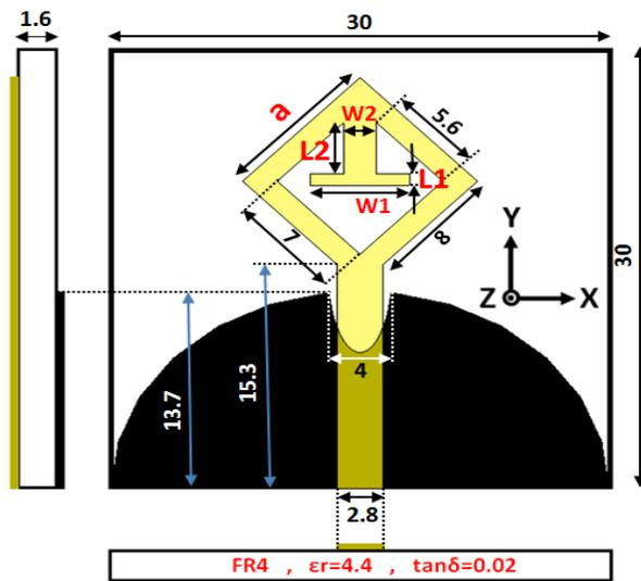
Fig. 1. Geometry of the proposed antenna (optimized dimensions in mm).
