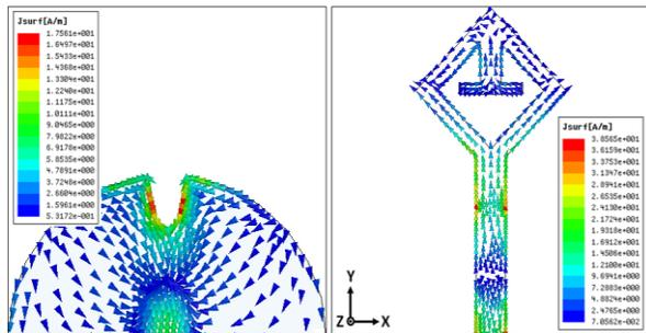
Fig. 9. Surface current distribution at 5.8 GHz over the defected ground-plane, feed-line and the patch.
