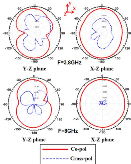
Fig. 7. Radiation patterns of the proposed antenna at: (a) 3.9 GHz, and (b) 8 GHz.
