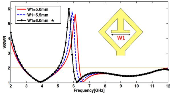
Fig. 3. Simulated VSWR characteristics of the proposed antenna for various dimensions of parameter  $W_1$ .
