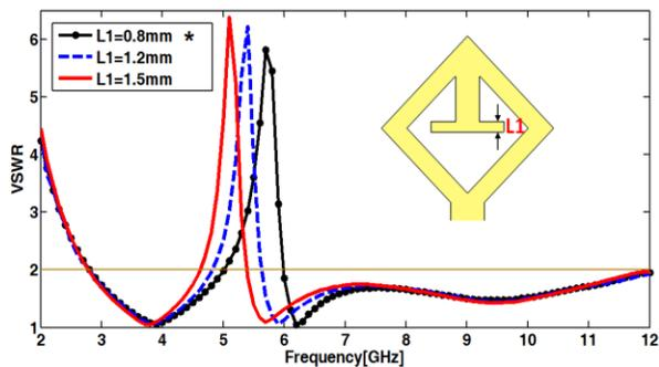
Fig. 5. Simulated VSWR characteristics of the proposed antenna for various dimensions of parameter  $L_1$ .
