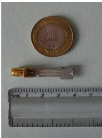
Fig. 11. SIW based ETS antenna without dielectric loading.
