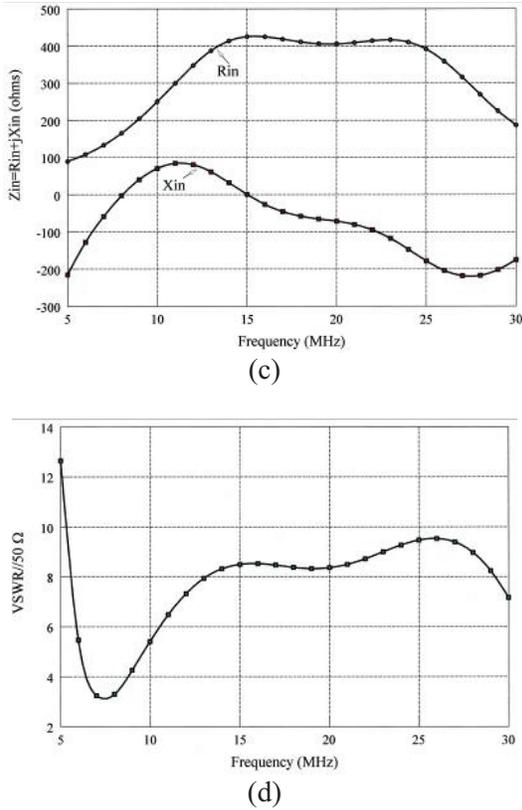
Fig. 8. Performance of monopole design # 3,  $f_3(502.5,7.214,50)$ .
