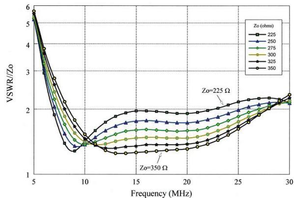
Fig. 11. VSWR for CFO design  $f_3(499.6,7.302,Z_0)$  parametric in  $Z_0$ .
