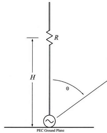
Fig. 1. Base-fed monopole geometry.
