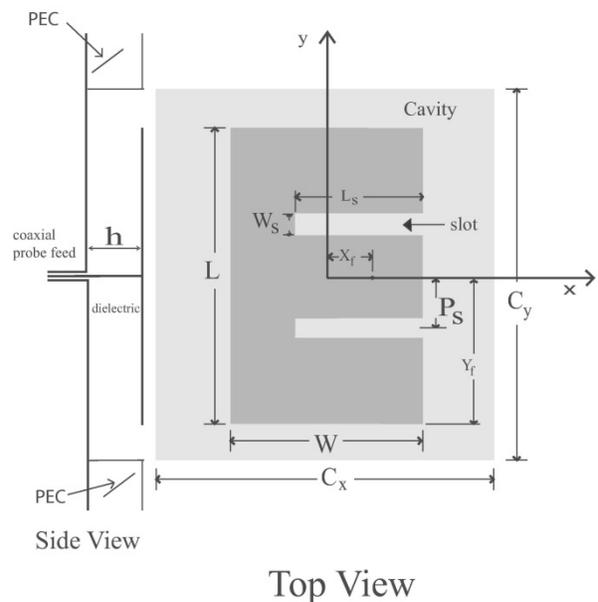
Fig. 1. Geometry of a planar cavity-backed E-patch antenna.
