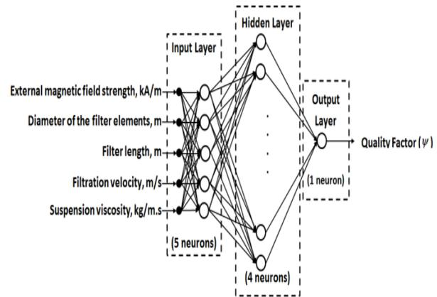
Fig.1. Schematic diagram of ANN model.
