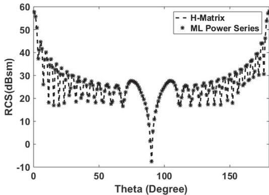
Fig. 2. Bi-static RCS of the PEC square plate with VV polarized plane wave incident at  $\theta = 0^\circ$ ,  $\phi = 0^\circ$ , and observation angles  $\theta = 0^\circ$  to  $180^\circ$ ,  $\phi = 0^\circ$ .
