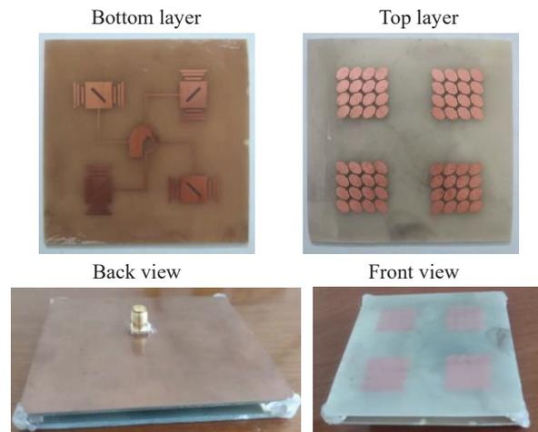
Fig. 9. Photos of the fabricated  $2 \times 2$  antenna arrays.
