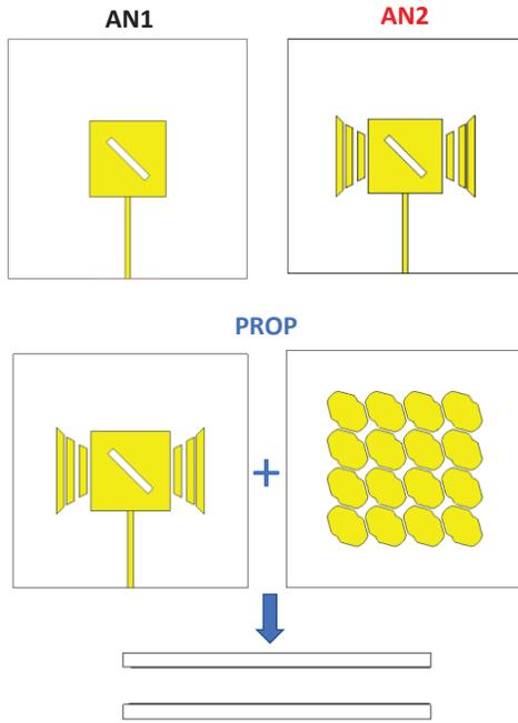
Fig. 4. Three different versions of the element antenna.
