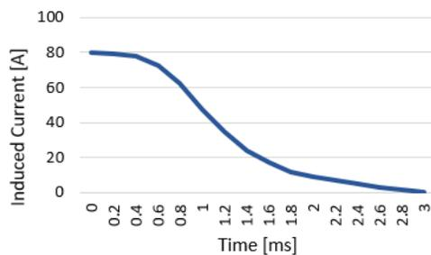
Fig. 8. Induced current in a rotor winding.
