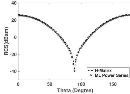
Fig. 3. Bi-static RCS of the dielectric slab with VV polarized plane wave incident at  $\theta = 0^\circ$ ,  $\phi = 0^\circ$ , and observation angles  $\theta = 0^\circ$  to  $180^\circ$ ,  $\phi = 0^\circ$ .
