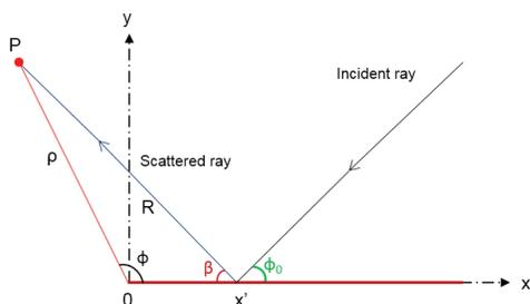
Fig. 1. Scattered beam geometry for the conductive half-plane.
