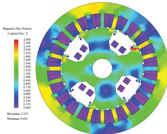
Fig. 9. Magnetic flux density plot of the machine.
