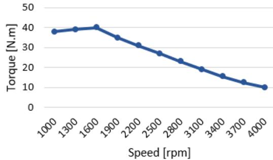
Fig. 19. Torque versus speed of the ISRM.
