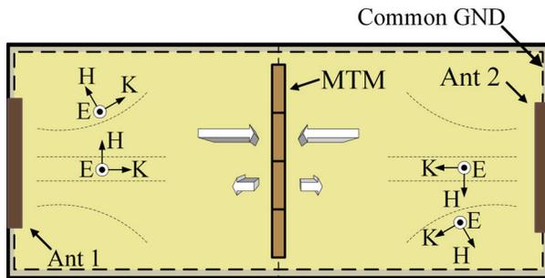
Fig. 3. Wi-Fi antenna system electromagnetic wave coupling schematic.
