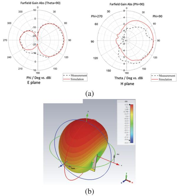
Fig. 4. The simulated and measured radiation pattern of Yagi Uda antenna (a) and 3D radiation pattern and (b) at 2.6 GHz.
