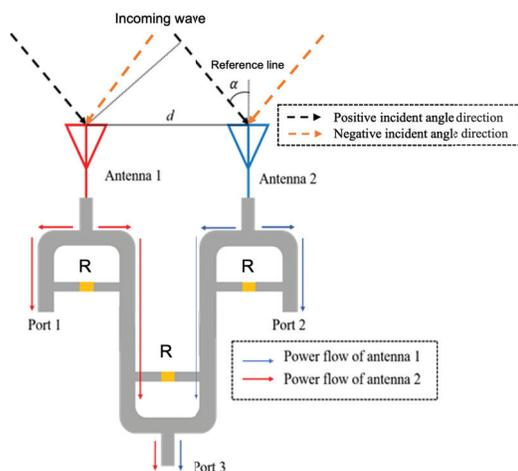
Fig. 2. The structure of DoA sensor unit.
