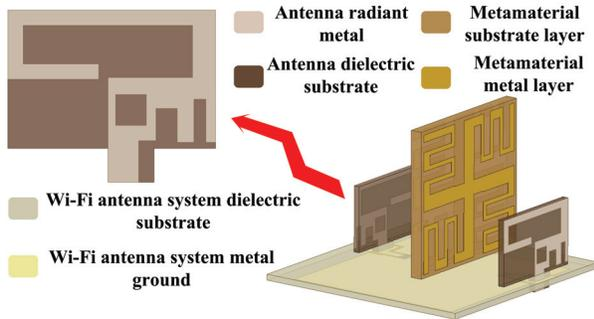
Fig. 1. Geometry structure of the antenna.
