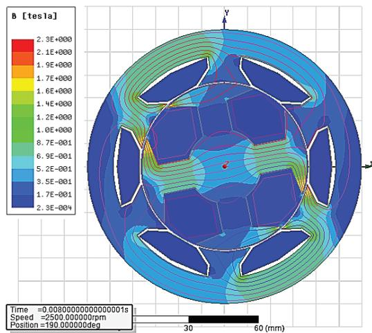
Fig. 2. Flux path in ISRM without rotor winding.
