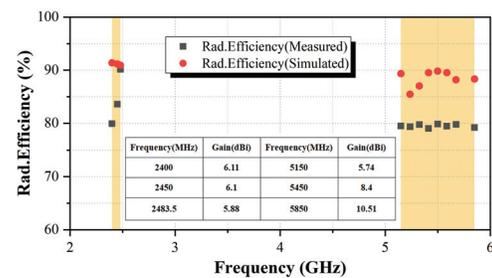
Fig. 12. Measured and simulated antenna efficiencies and gain.
