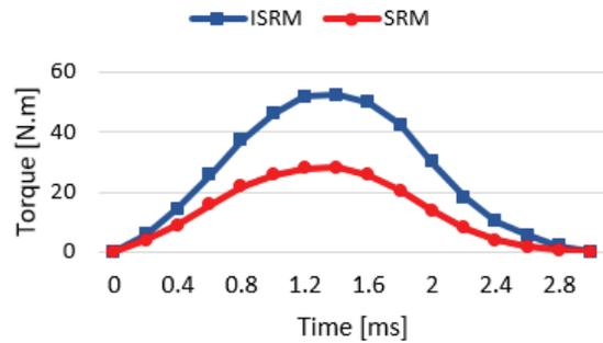
Fig. 5. Total torque of ISRM and SRM.
