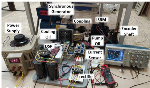
Fig. 14. The experimental setup of the ISRM.
