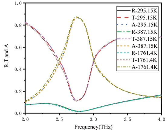
Fig. 4. Simulated reflection  $R$ , transmission  $T$ , and absorption  $A$  coefficients for the absorber, at temperature of  $295.15 \text{ K}$ , at temperature of  $387.15 \text{ K}$  and at temperature of  $1761.4 \text{ K}$ .
