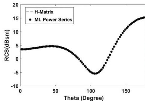
Fig. 4. Bi-static RCS of a dielectric hollow cylinder with VV polarized plane wave incident at  $\theta = 0^\circ$ ,  $\phi = 0^\circ$ , and observation angles  $\theta = 0^\circ$  to  $180^\circ$ ,  $\phi = 0^\circ$ .
