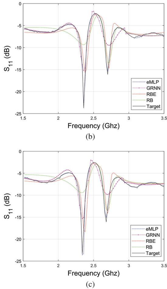
Fig. 6. Comparison of different ANN model performance parameter of the return loss ( $S_{11}$ ) of the antenna: (a)  $r=27$  (mm),  $w=1$  (mm),  $t=2.95$ , (b)  $r=27$  (mm),  $w=2.5$  (mm),  $t=2.6$ , and (c)  $r=27$  (mm),  $w=3$  (mm),  $t=2.60$ .
