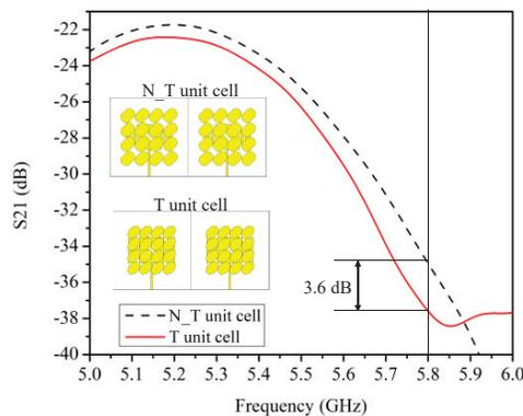
Fig. 7. Simulated  $S_{21}$  between two element antennas with the N-T unit cell and the T unit cell.
