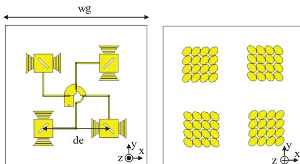
Fig. 8. The proposed  $2 \times 2$  antenna array.
