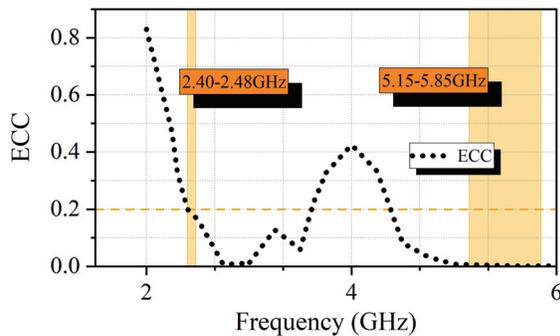
Fig. 15. The tested ECC at work frequency band.
