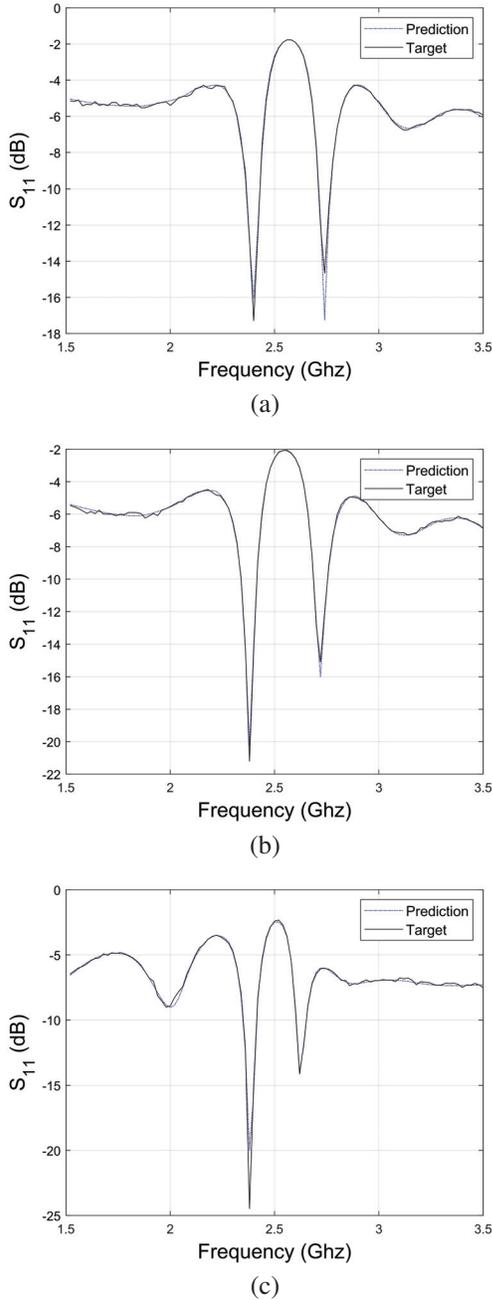
Fig. 5. eMLP model performance parameter of return loss ( $S_{11}$ ) for antenna: (a)  $r=27$  (mm),  $w=1.5$  (mm),  $t=2.6$ , (b)  $r=27$  (mm),  $w=2$  (mm),  $t=2.6$ , and (c)  $r=27$  (mm),  $w=2.5$  (mm),  $t=3.3$ .
