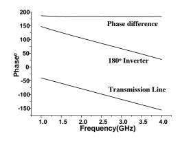
Fig. 7. Phase simulation of 180° inverter.
