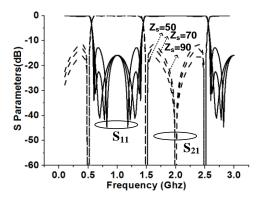
Fig. 3.  $S_{11}$  and  $S_{21}$  of circuit simulation.
