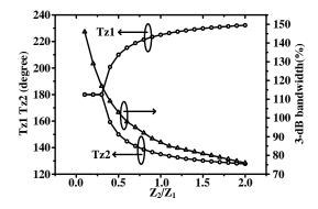
Fig. 2. Transmission zeros and the 3-dB bandwidth.
