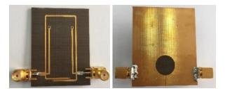
Fig. 10. Photograph of the proposed bandpass filter.
