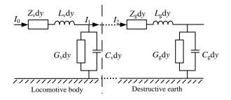
Fig. 4. Overhead line model equivalent circuit.
