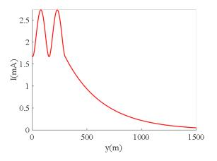
Fig. 7. Contact line current distribution curve.
