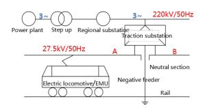
Fig. 1. Diagram of catenary power supply.
