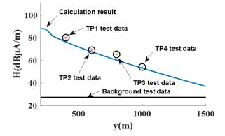
Fig. 8. Electromagnetic emission curve of the contact wire.
