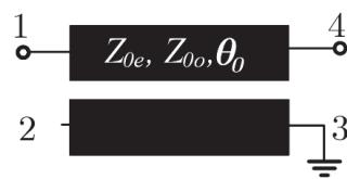
Fig. 2. Schematic of the proposed 2-port band stop filter based on parallel-coupled lines.
