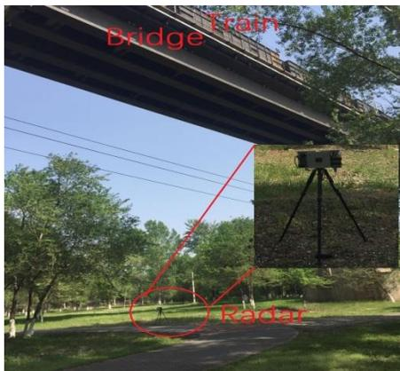
Fig. 7. Setup and scenario of freight railway bridge monitoring.
