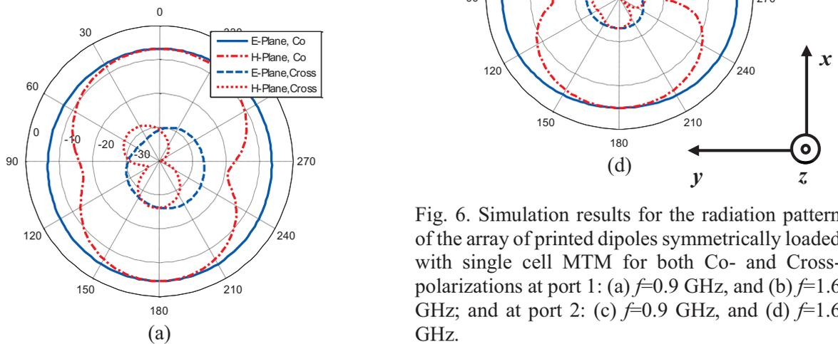
Fig. 6. Simulation results for the radiation pattern of the array of printed dipoles symmetrically loaded with single cell MTM for both Co- and Cross-polarizations at port 1: (a)  $f=0.9$  GHz, and (b)  $f=1.6$  GHz; and at port 2: (c)  $f=0.9$  GHz, and (d)  $f=1.6$  GHz.
