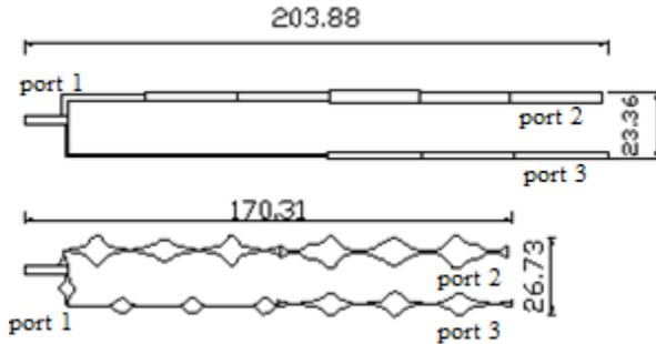
Fig. 9. The layout of the designed triple band NTL-based WPD compared to the conventional design (dimensions in mm).
