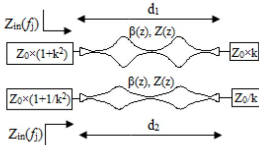
Fig. 3. Even-mode analysis of the unequal-split NTL-based WPD.
