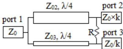
Fig. 1. A schematic of the conventional unequal-split WPD.
