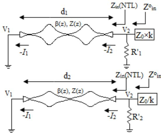
Fig. 4. Odd-mode analysis of the unequal-split NTL-based WPD.
