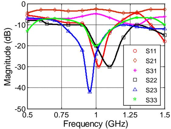
Fig. 7. Measured S-parameters of the fabricated NTL-based WPD.
