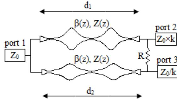
Fig. 2. A schematic of the unequal-split NTL-based WPD.
