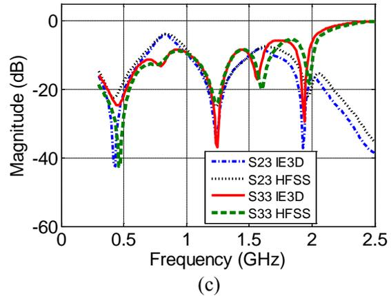
Fig. 10. S-parameters of the designed triple band NTL-based WPD.
