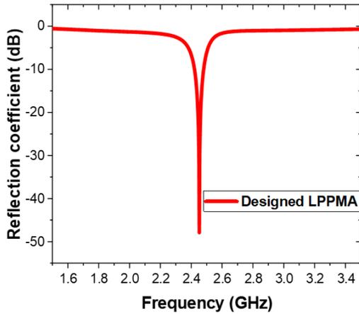
Fig. 20. Reflection coefficient of the designed LPPMA.
