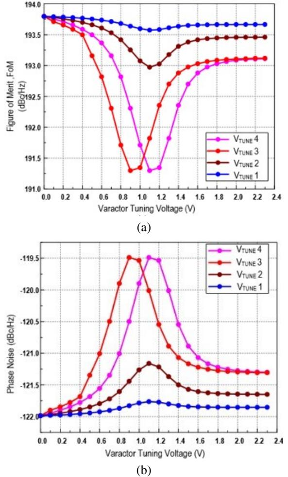
Fig. 10. Simulated performance of the dual core VCO (a) FoM and (b) PN performance across the varactor tuning voltages  $V_{TUNE1}$  -  $V_{TUNE4}$ .
