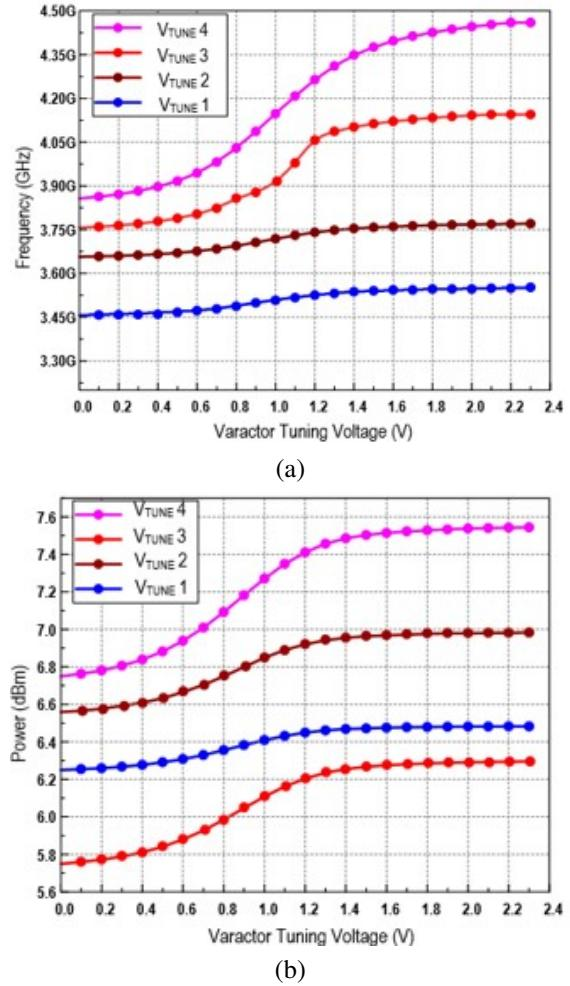
Fig. 13. Performance of the dual core VCO (a) frequency (GHz) and (b) output power (dBm) across the varactor tuning voltages  $V_{TUNE1}$ – $V_{TUNE4}$ .
