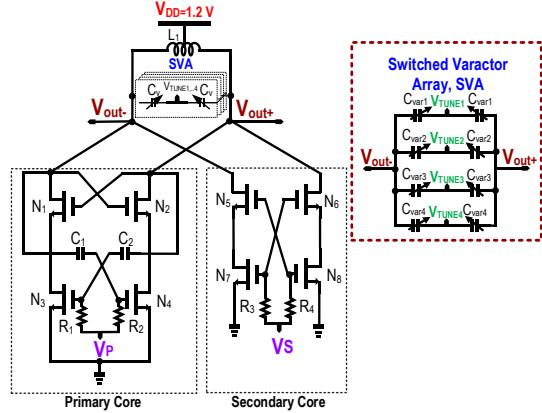
Fig. 2. Proposed LC-VCO with dual core VCO.
