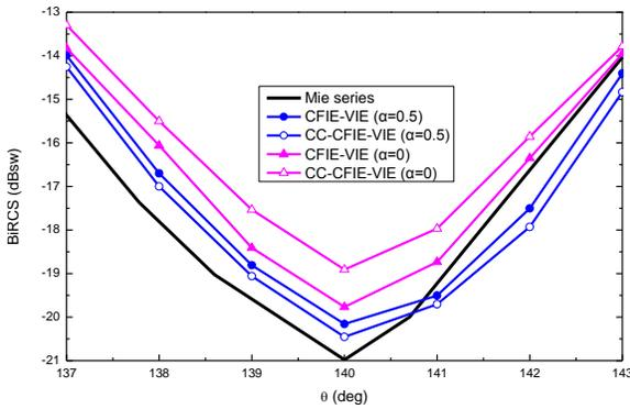
Fig. 4. Bistatic RCS of the coated PEC sphere at  $137^\circ \leq \theta \leq 143^\circ$  and  $\varphi=0^\circ$ , with 16 sampling points over the outer triangular integrations in the MFIE.
