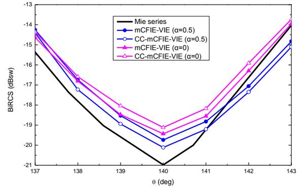
Fig. 5. Bistatic RCS of the coated PEC sphere at  $137^\circ \leq \theta \leq 143^\circ$  and  $\varphi=0^\circ$ , with the adoption of mMFIE.
