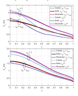
Fig. 5. Spatial coverage of the e-textile dipole (top) and e-textile folded dipole (bottom) at 915 MHz in the region where  $\theta = -90^{\circ}...90^{\circ}$  and  $\phi = -30^{\circ}...30^{\circ}$ .
