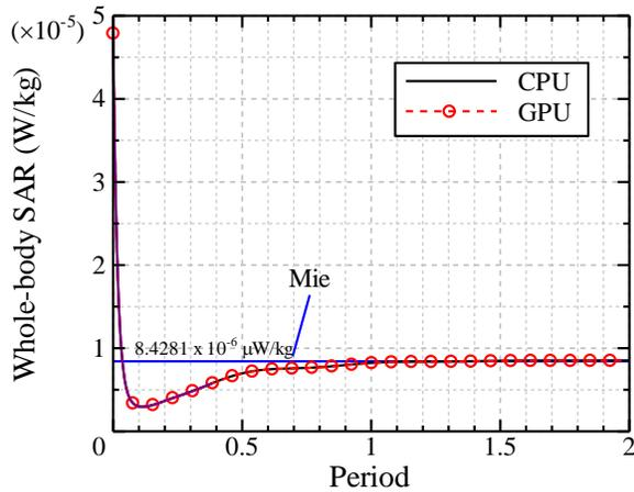
Fig. 5. Whole-body SAR of a dielectric sphere in time course, calculated by a workstation (24 parallel threads) and three GPUs (single node) on TSUBAME system.
