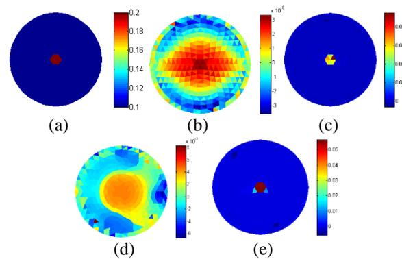
Fig. 3. The reconstructed results of model 2 with inhomogeneity in the centre. (a) Conductivity map, (b) the reconstructed image using  $L^2$  norm penalty, (c) the reconstructed image using the  $L^1$  norm penalty, (d) the reconstructed image using TV penalty, and (e) the reconstructed image using both  $L^1$  and TV penalties.
