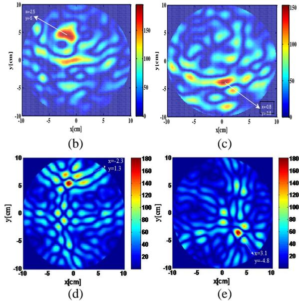
Fig. 10. (a) Experimental setup used to validate the proposed imaging system and the reconstructed images of the two tubes located at (b), (d)  $(-2,4)$  and (c), (e)  $(3.5, -4)$  coordinates first by a UWB transceiver (3.1-6.3 GHz frequency band), and then by using a Vector Network Analyzer (3.1-10.6 GHz frequency band).
