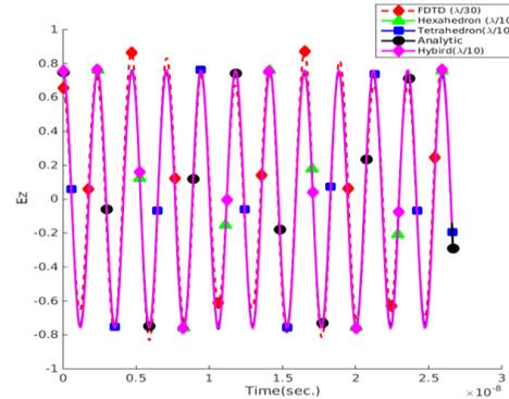
Fig. 4. Electric field distribution at point  $x=y=z=-0.167m$ .
