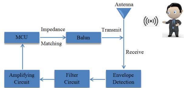
Fig. 1. Block diagram of our designed sensor.
