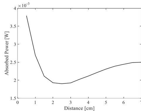
Fig 9. The absorbed power versus antennas separation distance.
