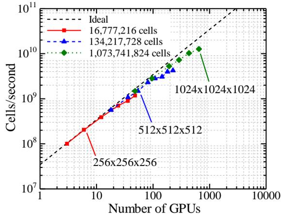
Fig. 7. Scalability for three problem sizes  $N = 256^3$ ,  $512^3$ , and  $1024^3$  on TSUBAME system at Tokyo Institute of Technology, Japan.
