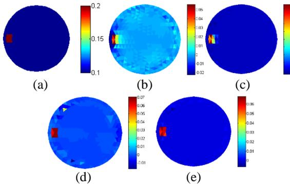
Fig. 2. The reconstructed results of model 1 with inhomogeneity near the boundary. (a) Conductivity map, (b) the reconstructed image using  $L^2$  norm penalty, (c) the reconstructed image using the  $L^1$  norm penalty, (d) the reconstructed image using TV penalty, and (e) the reconstructed image using both  $L^1$  and TV penalties.
