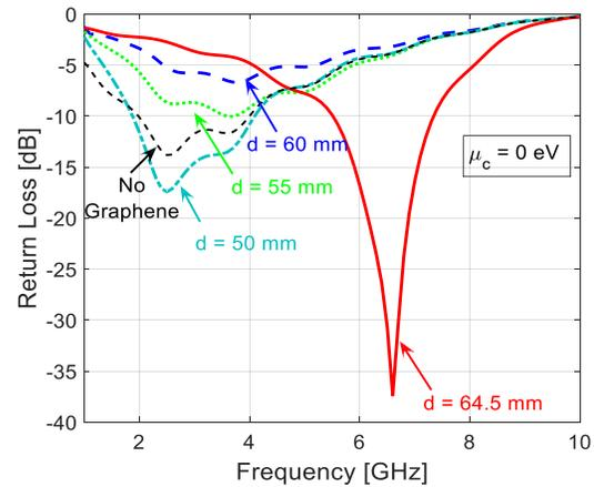
Fig. 7. Return loss obtained with the second configuration for different distances between the graphene and the slot.
