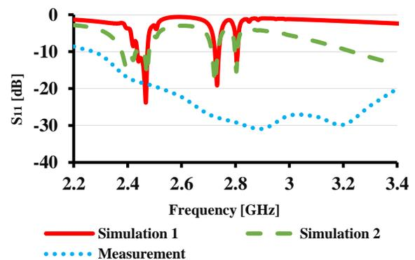
Fig. 7. Reflection coefficient of AMC antenna.
