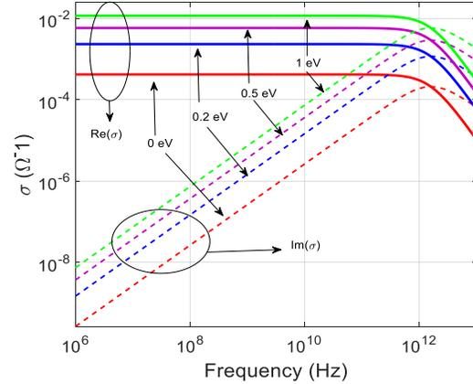
Fig. 1. Real and imaginary parts of the electrical conductivity of the graphene sheet as a function of the frequency for different values of the chemical potential.
