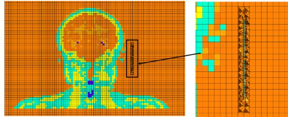
Fig. 1 Human head model exposed in dipole antenna.
