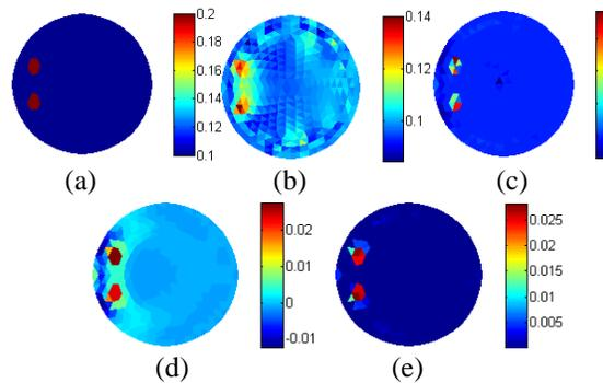
Fig. 4. The reconstructed results of model 3 with two small inclusions. (a) Conductivity map, (b) the reconstructed image using  $L^2$  norm penalty, (c) the reconstructed image using the  $L^1$  norm penalty, (d) the reconstructed image using TV penalty, and (e) the reconstructed image using both  $L^1$  and TV penalties.
