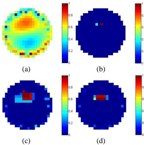
Fig. 8. The reconstructed current density images from the experimental magnetic field data. (a) The reconstructed image using  $L^2$  norm penalty, (b) the reconstructed image using the  $L^1$  norm penalty, (c) the reconstructed image using TV penalty, and (d) the reconstructed image using both  $L^1$  and TV penalties.
