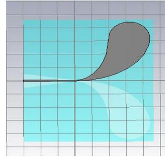
Fig. 3. Vivaldi antenna used in the proposed UWB imaging, each side of the square divisions is 1 cm.
