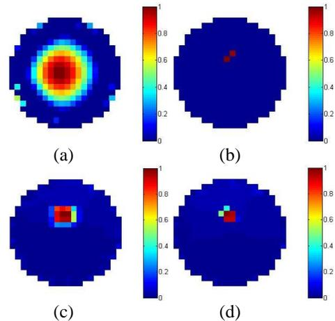
Fig. 7. The reconstructed current density images from the simulated magnetic field data with 50 dB white Gaussian noise. (a) The reconstructed image using  $L^2$  norm penalty, (b) the reconstructed image using the  $L^1$  norm penalty, (c) the reconstructed image using TV penalty, and (d) the reconstructed image using both  $L^1$  and TV penalties.
