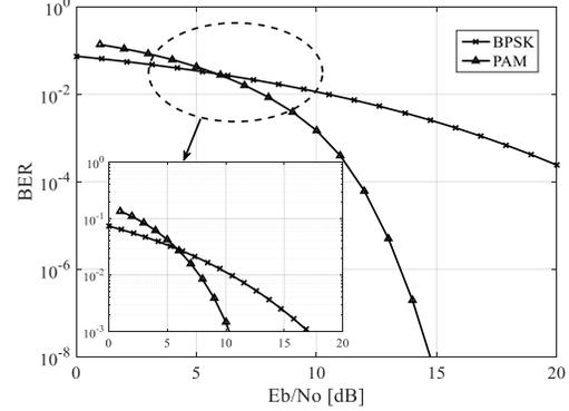
Fig. 10. SNR versus BER under the MIDA human head model fading channel under the BPSK and binary orthogonal PAM modulation schedules.
