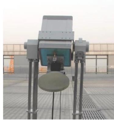
Fig. 2. A picture of the developed W-band radiometer.
