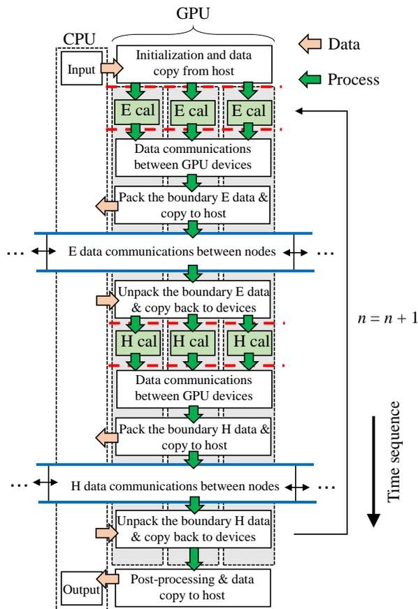
Fig. 4. Illustrative flowchart of the FDTD computation in a computing node. Dash line indicates synchronization between GPU devices (red dotted line) and MPI barrier between nodes (blue solid line).
