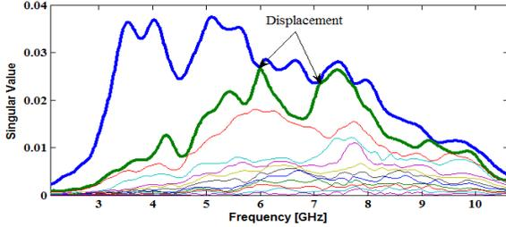
Fig. 1. Variations of singular values of two PEC spheres with different radii over the entire UWB frequency band.
