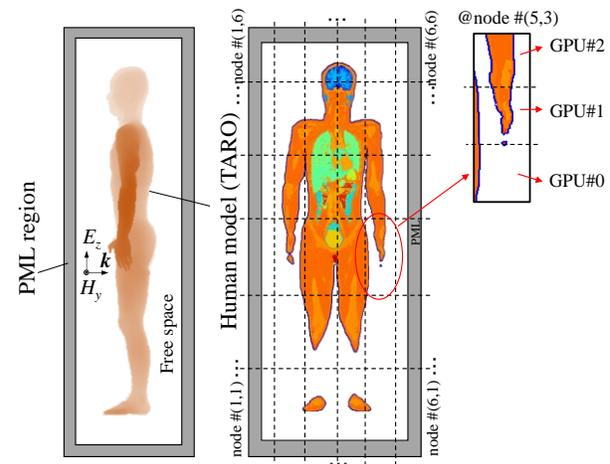
Fig. 8. Analysis model of EM exposure assessment of a realistic human model and the model decomposition into  $6 \times 6$  blocks in  $yz$ -plane. Each block corresponds to a computation node with three GPUs inside.
