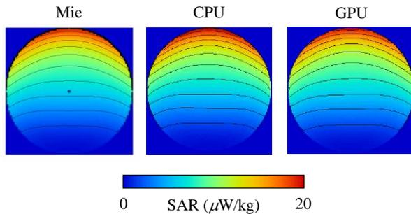
Fig. 6. SAR distribution of a dielectric sphere illuminated by a plane wave at 200 MHz, by the Mie's solution, and those obtained from the CPU and GPU computations.
