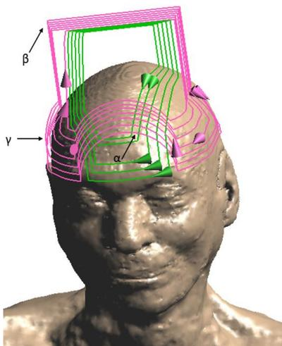
Fig. 1. Front view of H1 coil positioning on the head of model Glenn with the indication of the three portion described in the text: base portion ( $\alpha$ ), protruding return portion ( $\beta$ ), and contacting portion ( $\gamma$ ).
