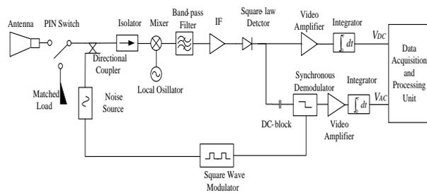
Fig. 1. Block diagram of the radiometer receiver.
