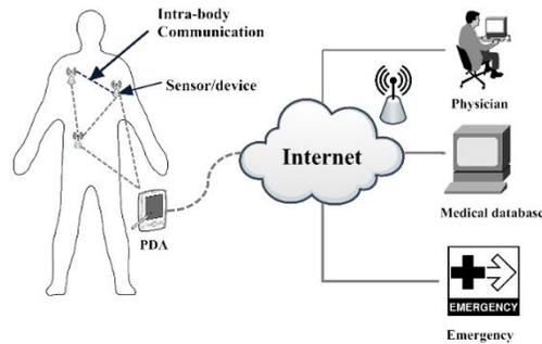
Fig. 1. Typical architecture of an implant WBAN system.
