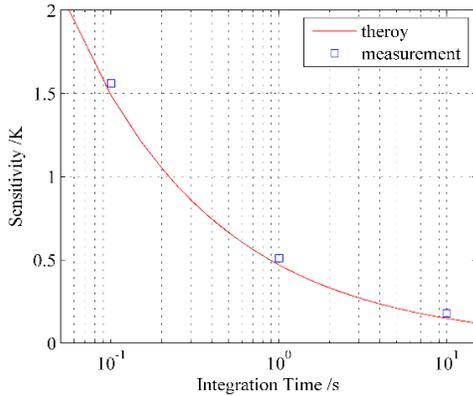
Fig. 4. The radiometer sensitivity with different integration time.
