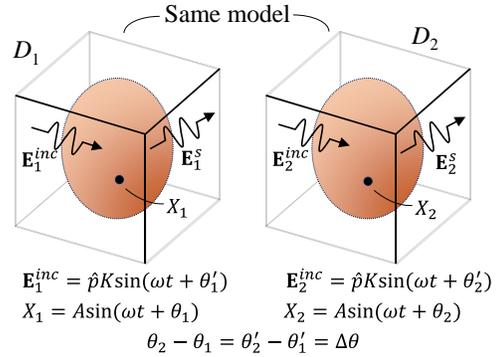
Fig. 1. Concept of an approach for determination of the whole-body average SAR in time course by defining two identical problem domain  $D_1$  and  $D_2$  with an incident field having a constant phase difference of  $\Delta\theta = \theta_2' - \theta_1'$ .  $K$  and  $A$  are the magnitude of the incident electric field  $\mathbf{E}_{1,2}^{inc}$  and the FDTD-calculated field of the solution, respectively,  $\hat{p}$  is the polarization vector.
