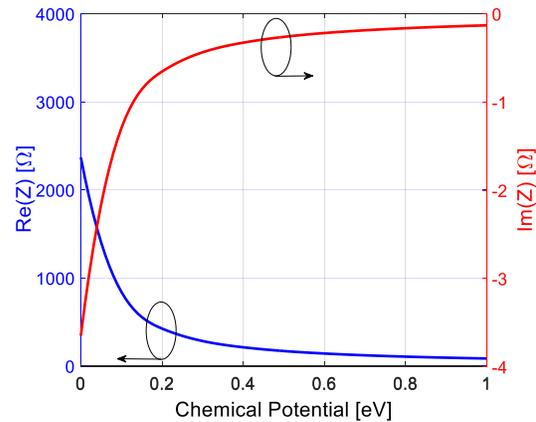
Fig. 2. Resistance and the reactance of the surface impedance of a graphene sheet as functions of the chemical potential.
