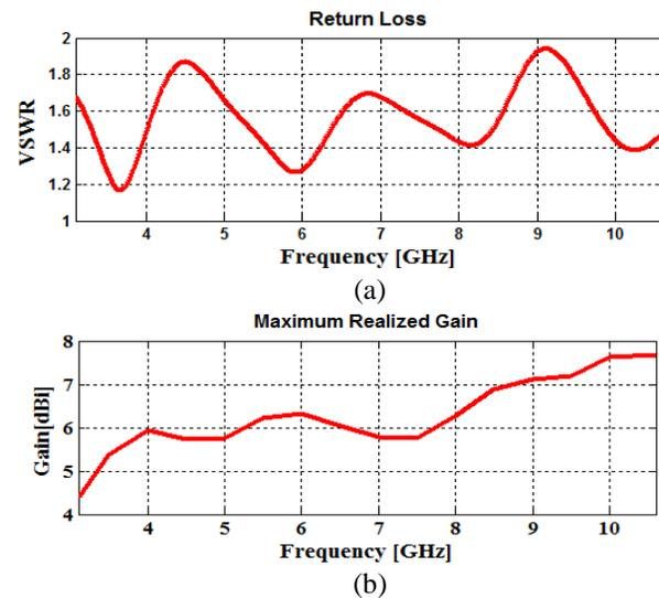
Fig. 4. Simulated (a) VSWR and (b) maximum gain of the UWB antenna.
