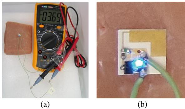
Fig. 4. Photograph of the LED light-up demonstration for the rectenna: (a) photograph of the LED light-up demonstration, and (b) enlarged photograph of the wirelessly lit LED in the rectenna.
