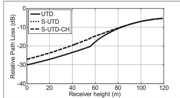
Fig. 3. Comparison of the results for hard polarization.
