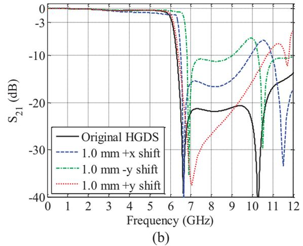
Fig. 4. Comparison of simulated  $S_{21}$  between the original proposed low-pass filter design (solid line) and spatial sensitivity test cases: (a) 0.5-mm displacements in HGDS designs and (b) 1.0-mm displacements in HGDS designs.
