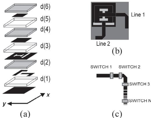
Fig. 3. Dual-polarization reflectarray element based on patches aperture-coupled to delay lines. (a) Expanded view. (b) Upper view. (c) Implementation of series switches in the delay line.
