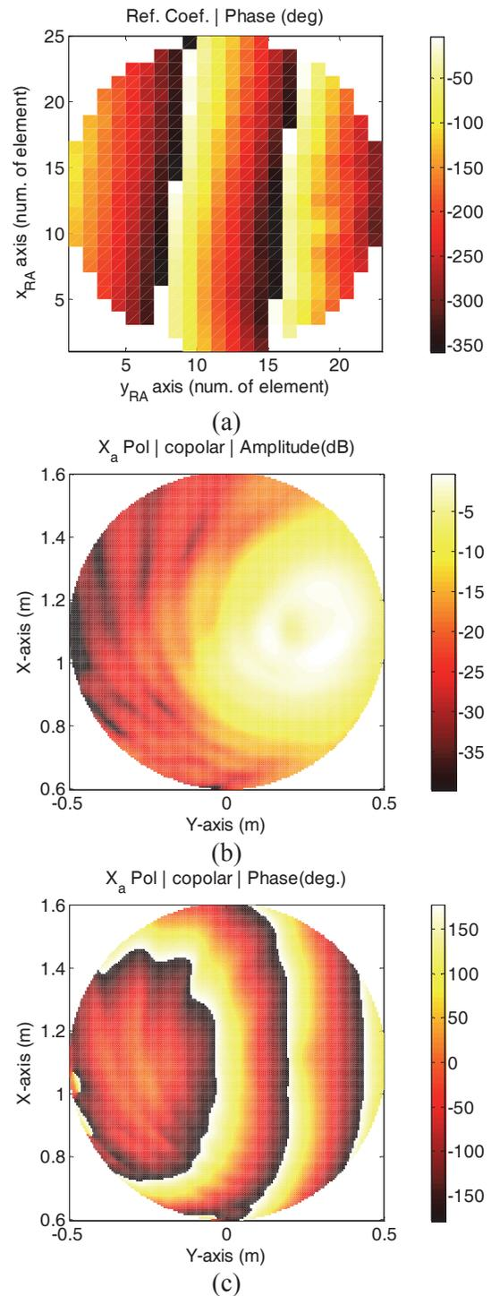
Fig. 6. Case of  $+6$  degree deflected beam in azimuth with continuous phase-shift control. (a) Required phase shift of the sub-reflector array. (b) Amplitude and (c) phase of the electric field at the antenna aperture.
