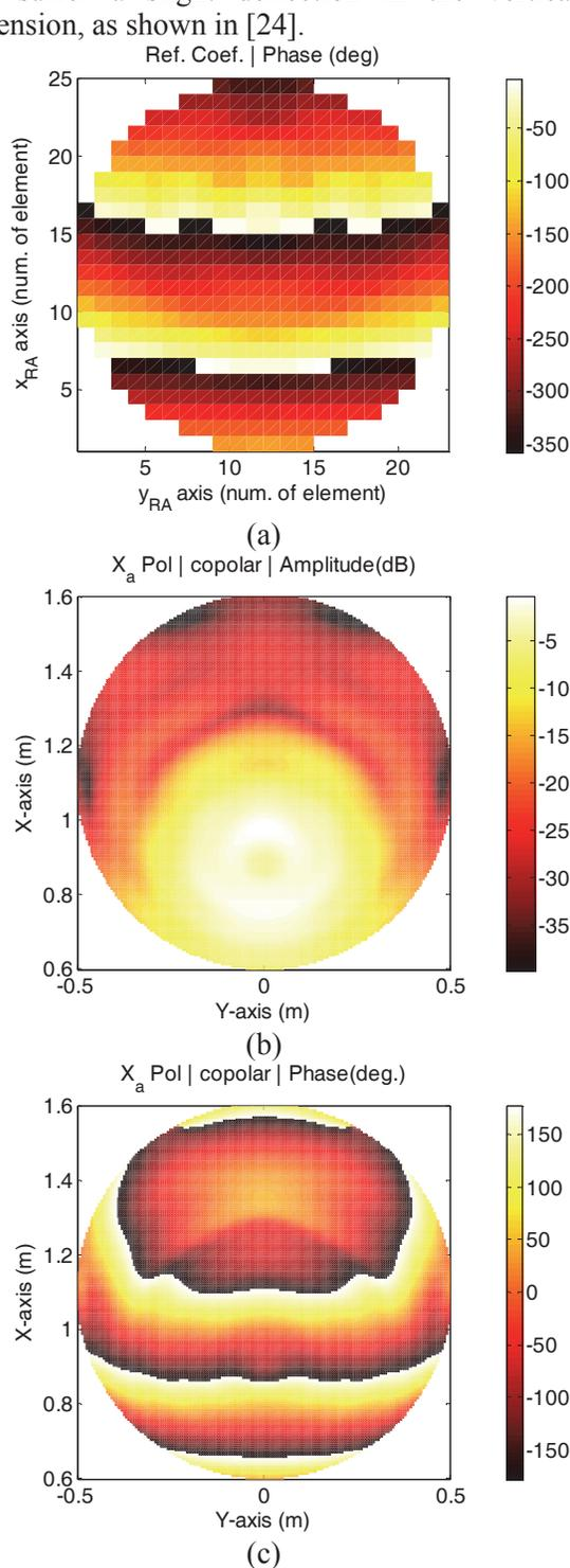
Fig. 5. Case of  $-6$  degree deflected beam in elevation with continuous phase-shift control. (a) Required phase shift of the sub-reflector array. (b) Amplitude and (c) phase of the electric field at the antenna aperture.
