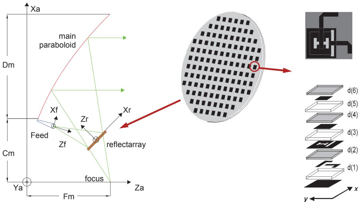
Fig. 1. Scheme of the dual-reflector configuration.
