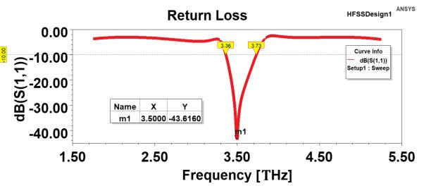
Fig. 4. Simulated return loss value at 3.5 THz.
