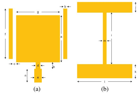
Fig. 3. Proposed 3.5 THz MPA structure: (a) radiating layer, (b) bottom layer.
