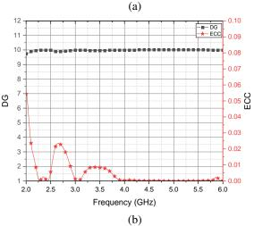
Fig. 8. ECC and DG versus frequency plot of MIMO RDRA: (a) without the slotted ground, and (b) with the edged hole and slotted ground.
