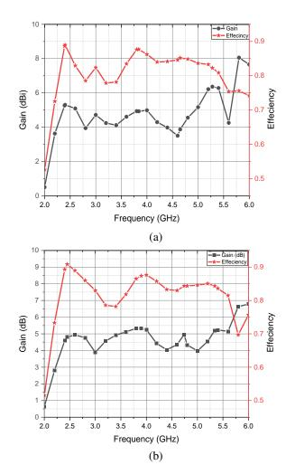
Fig. 7. Gain and radiation efficiency of MIMO RDRA: (a) without, and (b) with an edged hole and slotted ground.
