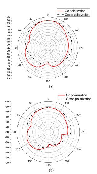
Fig. 5. MIMO RDRA antenna's simulated radiation pattern (without the edged hole and slotted ground): (a) Eplane Co and cross-polarization dB (V/m) at 2.39 GHz, and (b) H-plane Co and cross-polarization dB (A/m) at 2.39 GHz.
