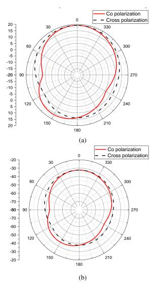
Fig. 6. MIMO RDRA antenna's simulated radiation pattern (with edged hole and with slot): (a) E-plane Co and cross-polarization dB (V/m) at 2.4 GHz, and (b) H-plane Co and cross-polarization dB (A/m) at 2.4 GHz.
