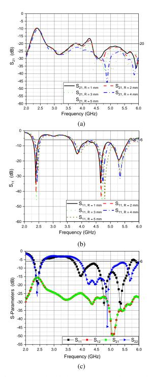
Fig. 3. MIMO edged hole RDRA: (a)  $S_{21}$ , (b)  $S_{11}$  as the hole radius varies, and (c) S-parameters with the slotted ground plane.
