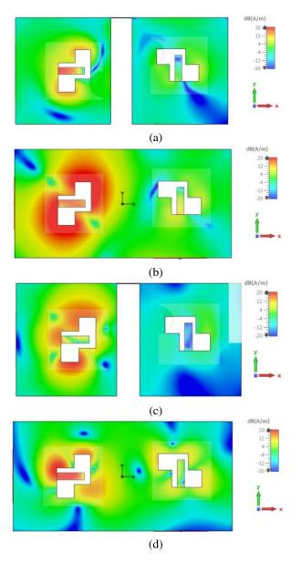
Fig. 4. Surface current distribution of MIMO RDRA: (a) with edged hole and slotted ground at 2.4 GHz, (b) without the edged hole and slotted ground at 2.4 GHz, (c) with edged hole and slotted ground at 4.2 GHz, and (d) without the edged hole and slotted ground at 4.2 GHz.
