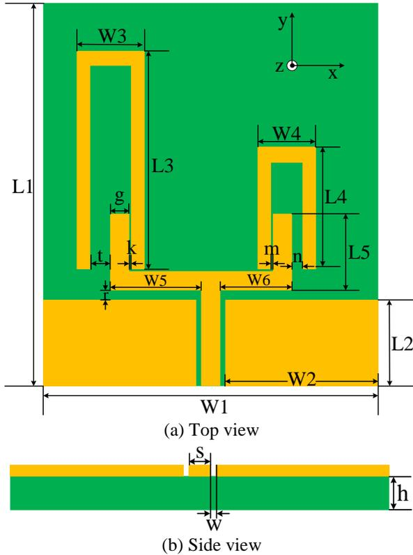
Fig. 1 Geometry structure of the proposed antenna.
