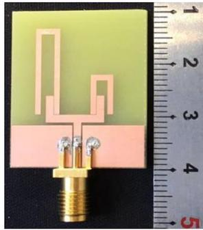
Fig. 3. Photograph of the fabricated dual-band WLAN antenna.
