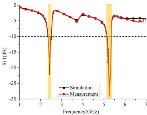
Fig. 4.  $S_{11}$  of the proposed dual-band antenna.
