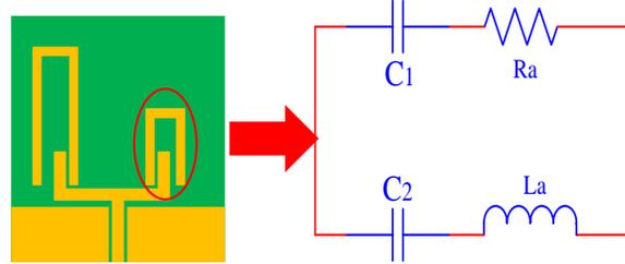
Fig. 2. Equivalent circuit of inverted U-shaped reactive loading.
