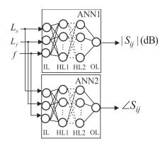
Fig. 2. ANN model of RF MEMS switch S-parameters.
