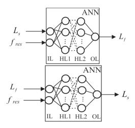
Fig. 5. ANN based determination of RF MEMS switch geometrical parameters.
