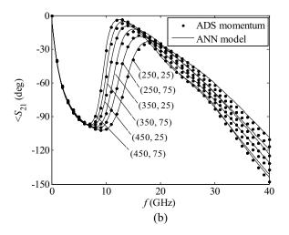
Fig. 7. Parameter  $S_{21}$  for six  $(L_s \, [\mu m], L_f \, [\mu m])$  combinations not used for the model development: (a) magnitude and (b) phase.
