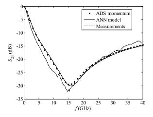
Fig. 8. Isolation of the fabricated RF MEMS switch  $(L_s = 174 \ \mu \text{m} \text{ and } L_f = 40 \ \mu \text{m}).$
