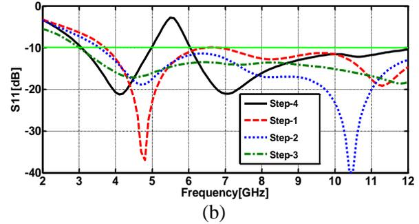
Fig. 2. (a) Simulated VSWR and (b) S11 characteristics for four steps used to create the proposed antenna structure.
