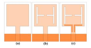
Fig. 2. (a) Basic structure (a square monopole antenna with a ground etch), (b) the antenna with a pair of rotated T-shaped slots and (c) antenna with a pair of rotated T-shaped slots and a pair of L-shaped conductor-backed plane.
