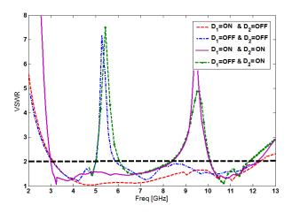
Fig. 9. Measured VSWR characteristics for the proposed antenna.
