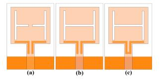
Fig. 5. Various structures for the proposed reconfigurable antenna: (a)  $D_1=ON \& D_2=OFF$ , (b)  $D_1=OFF \& D_2=OFF$  and (c)  $D_1=OFF \& D_2=ON$ .
